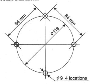
The tower plate onto which the rotator unit is mounted must be drilled with four holes of 9 mm diameter, equally spaced on a circle of 119 mm diameter. The center-to-center distance between any two adjacent mounting holes is 84 mm.
