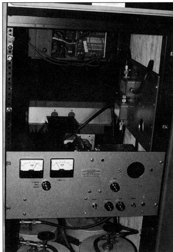
Figure 4—An inside view of the WIKKF repeater. The controller takes center stage, while the duplexer is visible at the bottom of the cabinet.
