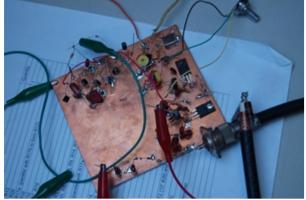
Figure 2. Measuring output power with my vintage VOM. Variable capacitor (near the top of photo) for the VXO was salvaged from an old tube AM radio. Output being measured during testing is about 50 mW.
