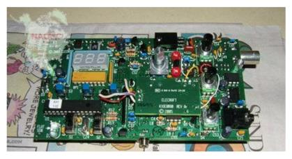
Finally after some time, we got the KB3080 board finished and mounted on the main KX-1 board as shown here. With our replacement vari-colored wires, we figure we must have one of the most colorful KX-1's around. We made the checks in the manual to be sure everything was working up to this point and it was.
