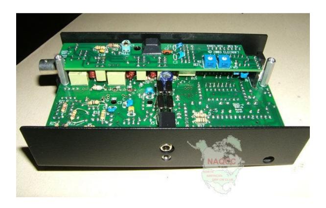
A check-out of the tuning unit started with a vivid demonstration. When Mike put on the phones to listen and turned on the rig, he was blasted with a great increase in volume over what it was with just a jumper in place of the ATU. After he recovered from that blast we continued. The check-out procedure showed that all of the relays in the ATU were functioning perfectly.
