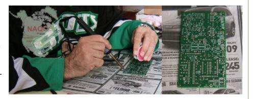
A couple members expressed concern that we weren't doing enough to prevent static damage to sensitive parts. While not apparent from the photos, the card tables we are working on have a metal frame that acts as a very good ground as we are in contact with it most of the time. When we get to an extra sensitive part, we also touch the frame several times while working with it as an extra precaution.
