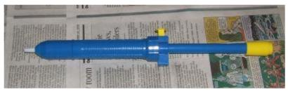
Always have a very good solder sucker while building the KX-1 or any kit. One of the easiest ways to damage a PC board is desoldering and re-soldering a connection. A good solder sucker allows the process to take place
