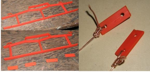
To extend the 10 meter dipole to 20 meters we needed two 8 feet 4 inches segments. We connected those to the insulators at the ends of the 10 meter dipole with the end of the wire bared so we could connect the alligator clip to it, thus making a 20 meter dipole.
