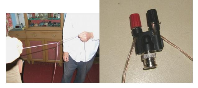
At each end of the dipole we put an insulator made from end pieces of the extension cord wrapper and connected an alligator clip to the end of the wire. The pupose being to have a point where we could connect another segment of wire for 20 meters.
