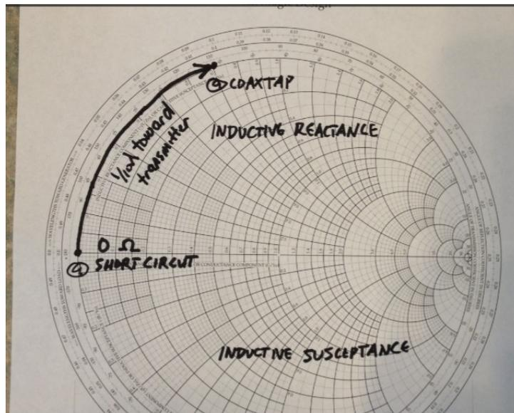
*Shorted section has 0 ohms at its shorted end, but 1/10 wavelength away it has considerable inductance, which is in parallel with the coaxial feed.*
