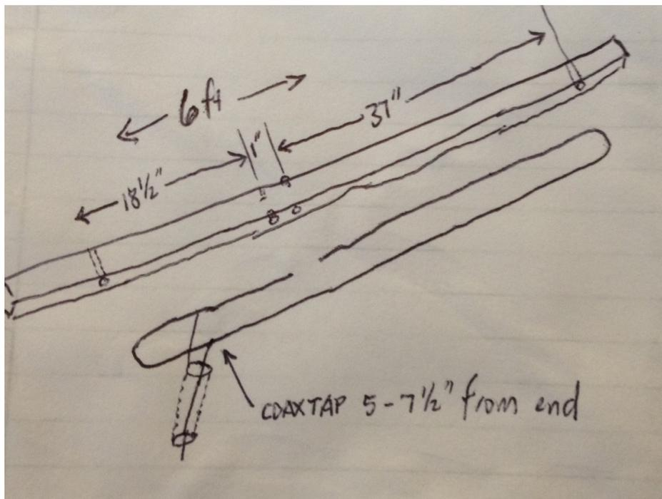
*Drawing of the wood and wire that make up the antenna. The end-fed folded dipole is the longer, righthand portion, while the transmission line matching network is the left hand portion of the wire to which the coax is attached.*
