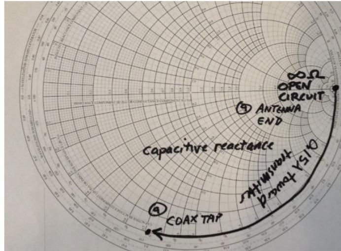
Seemingly “open-ended” balanced line section has near infinite ohms (near open circuit, because the end impedance of a  $\frac{1}{2}$  wave dipole is very very high, and the second wire of the feedline goes NOWHERE) but 0.15 wavelengths back toward the transmitter (at the coax feed point) it has significant capacitance – which is effectively “in-line” (in series) with the antenna.
