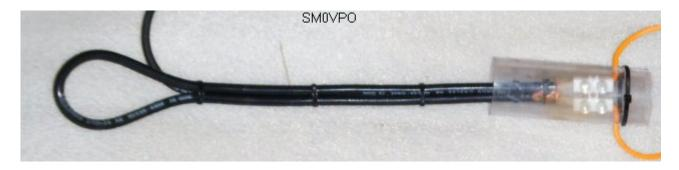
The completed balun feeding the antenna.
