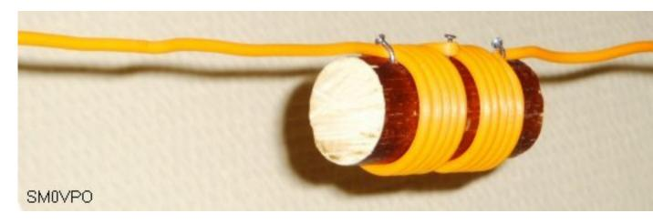
The finished stub positioned in the antenna wire.
