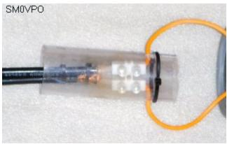
The connector feeding the antenna elements.
