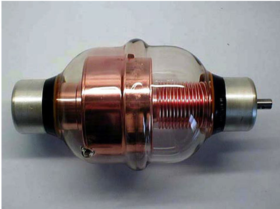
Figure 3 Large kVA / VAR rated vacuum variable capacitor
