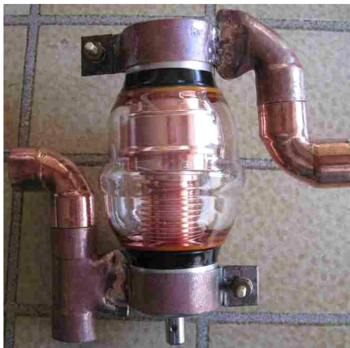
Figure 16 Homebrew capacitor clamps with silver-soldered copper fittings
