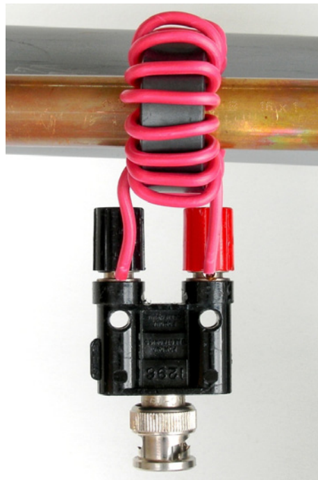
Figure 12 Conceptual and practical realisation of transformer coupling
