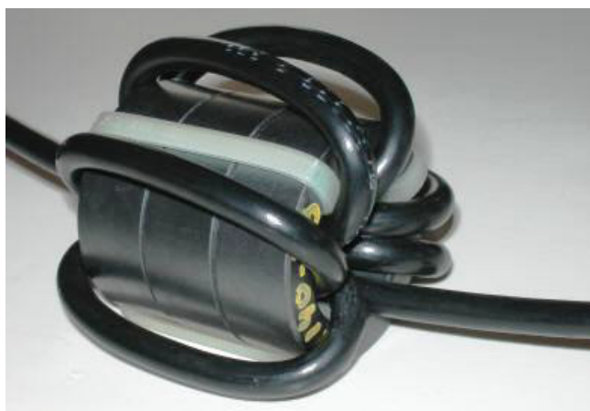
Figure 9 Alternative common-mode choke construction
