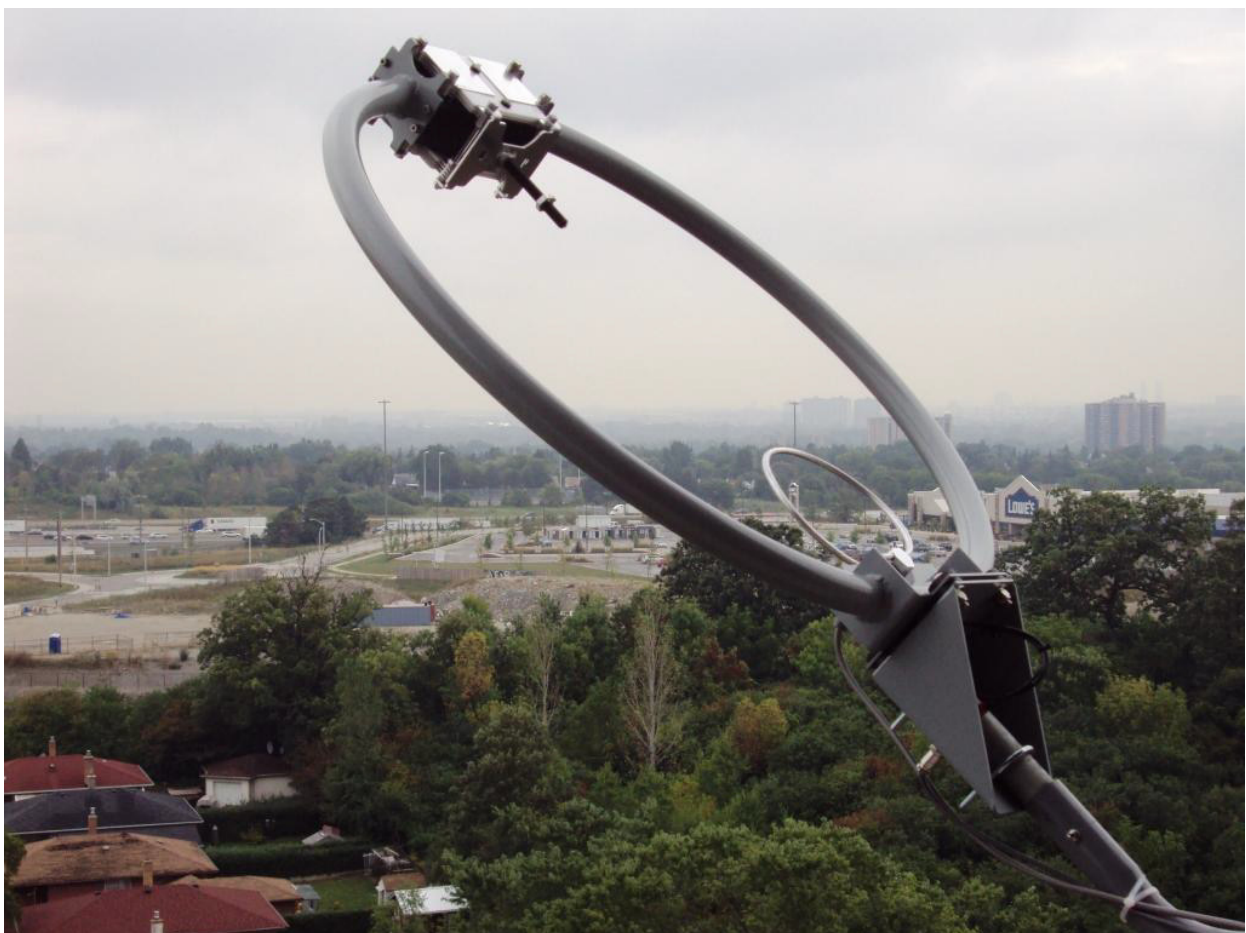
Figure 22 An MLA deployment on elevated condominium balcony
