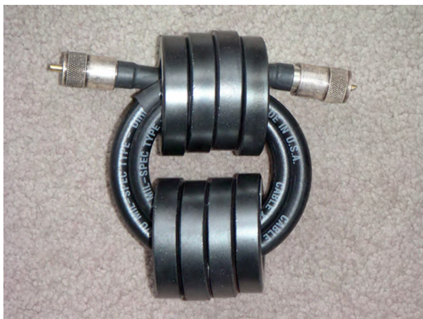
Figure 7 Multi-turn high power common-mode choke balun
