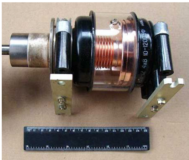
Figure 17 Russian Mil-style vacuum variable with integral clamps
