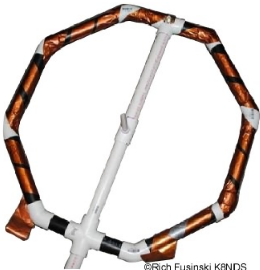
Figure 6A: Flat conductor loop (helically wound/loaded, shown without capacitor) and Slinky™ coil loop (sources: ref. 5A/B and 5C)
