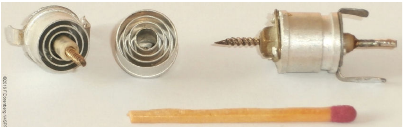
Figure 14: Philips tubular-piston "beehive" trimmer capacitors (5-30 pF, 0.3 mm plate distance)
