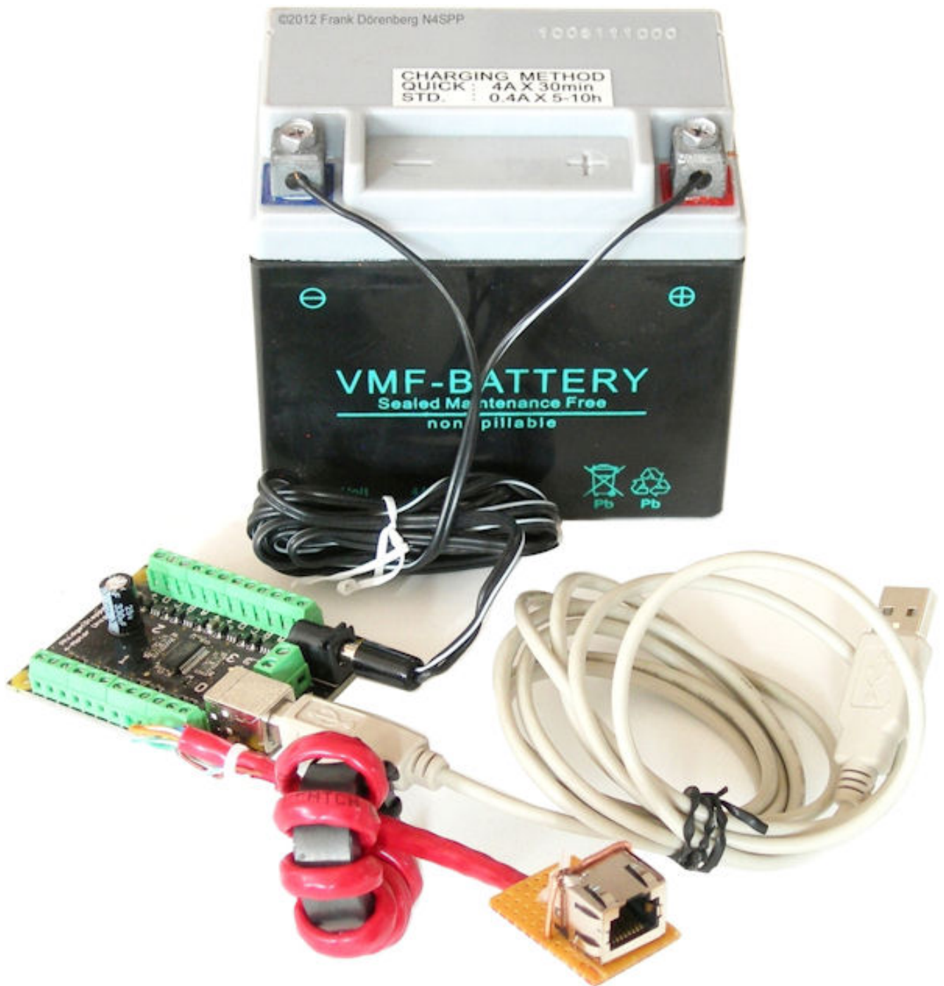
Fig. 102: Toroidal current choke on the CAT5 cable between controller card and stepper-motor
