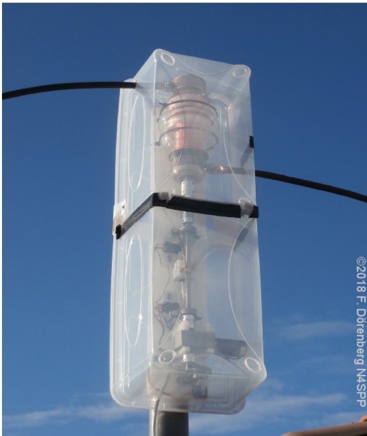
Figure 122: Weather protection Mk 1 - installed
