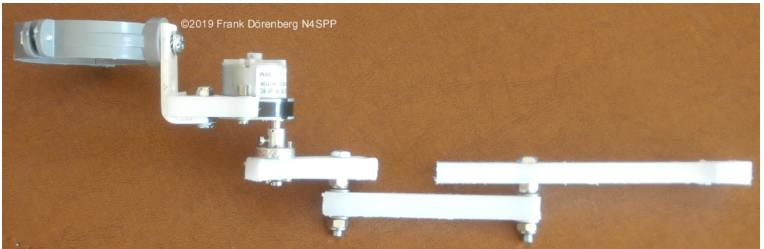
Figure 139: Side view of the double-eccentric drive for the coupling loop
