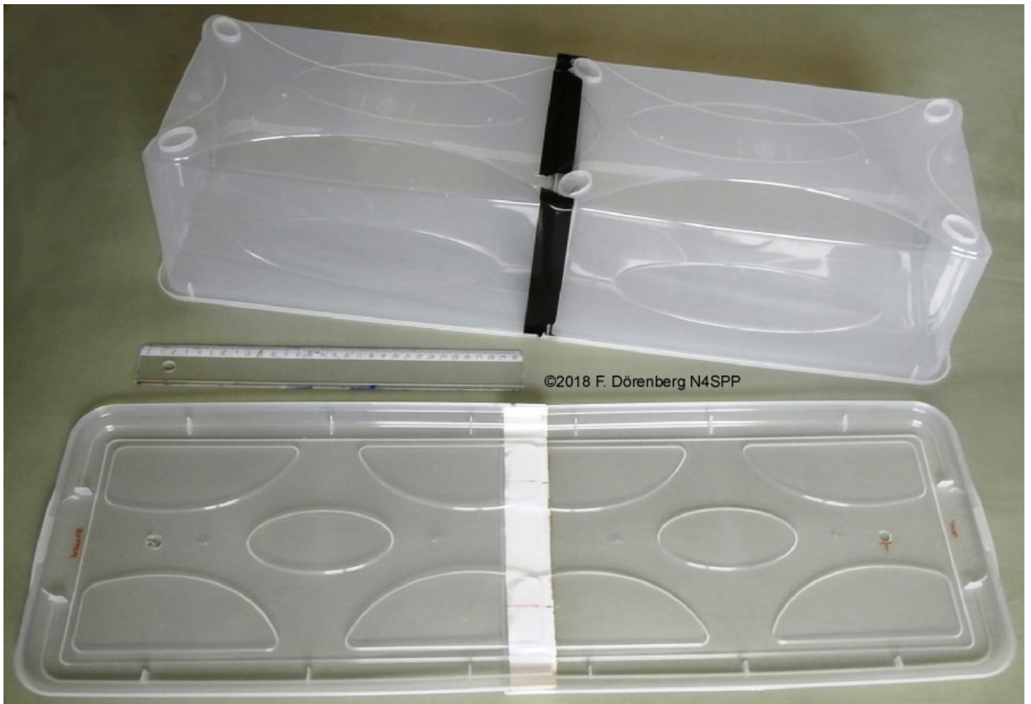
Figure 121: Protective hood made of two clear plastic boxes and their lids
