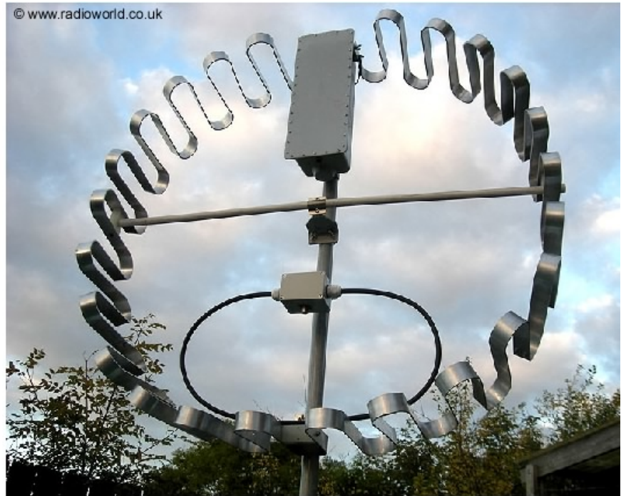
Figure 6B: Flat conductor loop and meandering "fractal" loop (source: ref. 4 and www.radioworld.co.uk )
