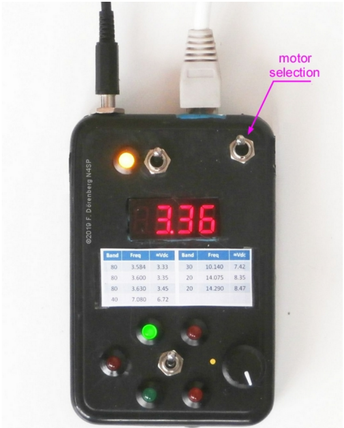
Figure 144: The remote control box - now with a toggle switch for motor selection
