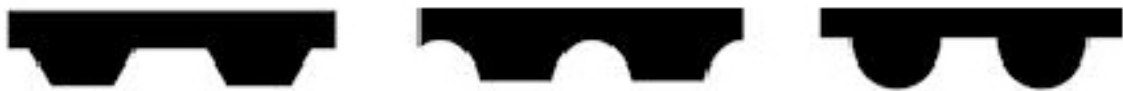
Figure 95: Standard metric belt profiles (left to right: T, AT, HDT) (similar British/Imperial profiles are L, H, XL, MXL)
