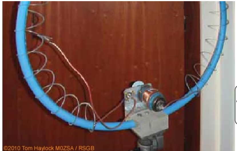
Figure 6A: Flat conductor loop (helically wound/loaded, shown without capacitor) and Slinky™ coil loop (sources: ref. 5A/B and 5C)
