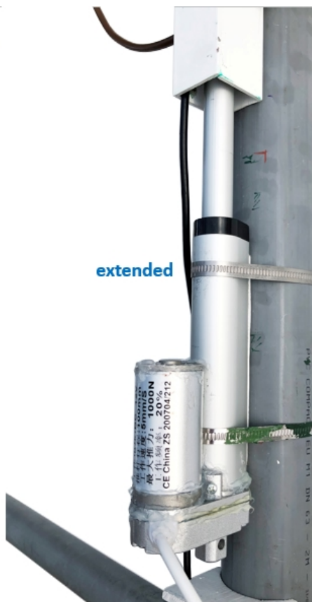
Fig. 148: My coupling with linear motor drive
