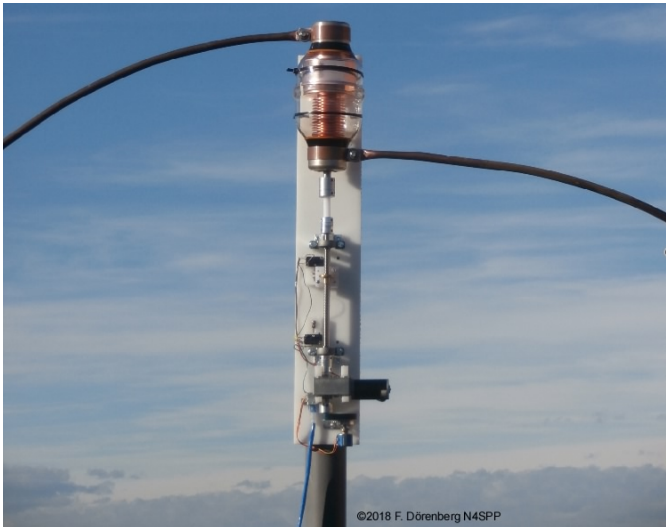
Figure 120: Motor drive installed on the PVC-tube antenna mast
