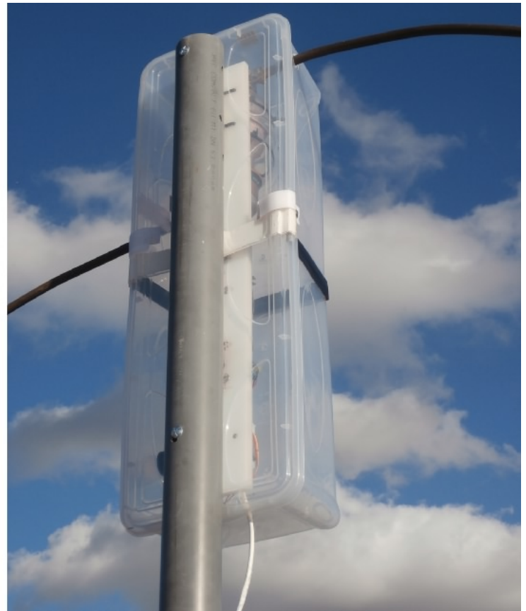
Figure 122: Weather protection Mk 1 - installed
