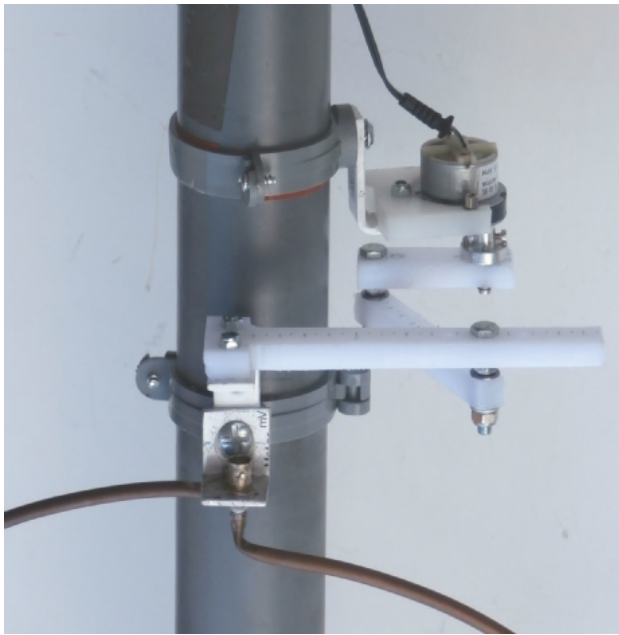
Figure 141: the double-eccentric drive for the coupling loop - installed
