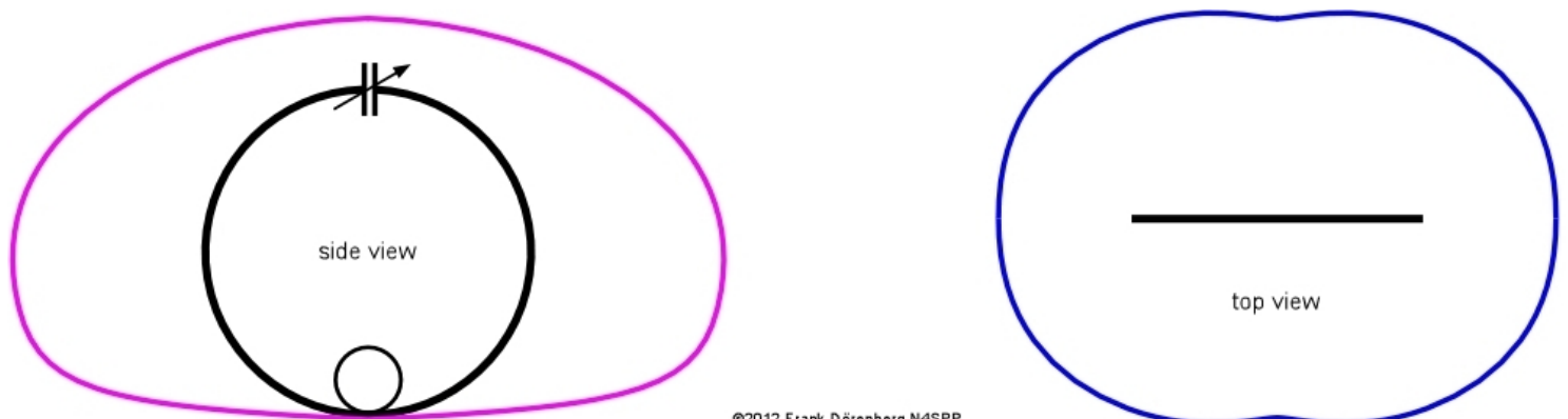
Fig. 2: approximate radiation pattern of a vertically oriented Small Transmitting Loop close to ground
