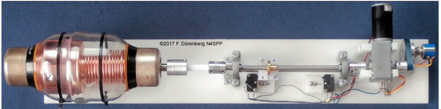
Figure 113: Top view of the DC motor drive assembly with vacuum capacitor
