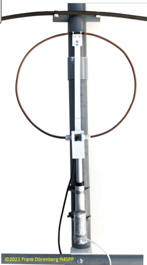
Fig. 148: My coupling with linear motor drive
