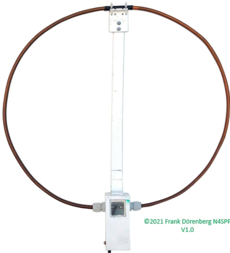
Fig. 147: My new coupling loop with mounting box
