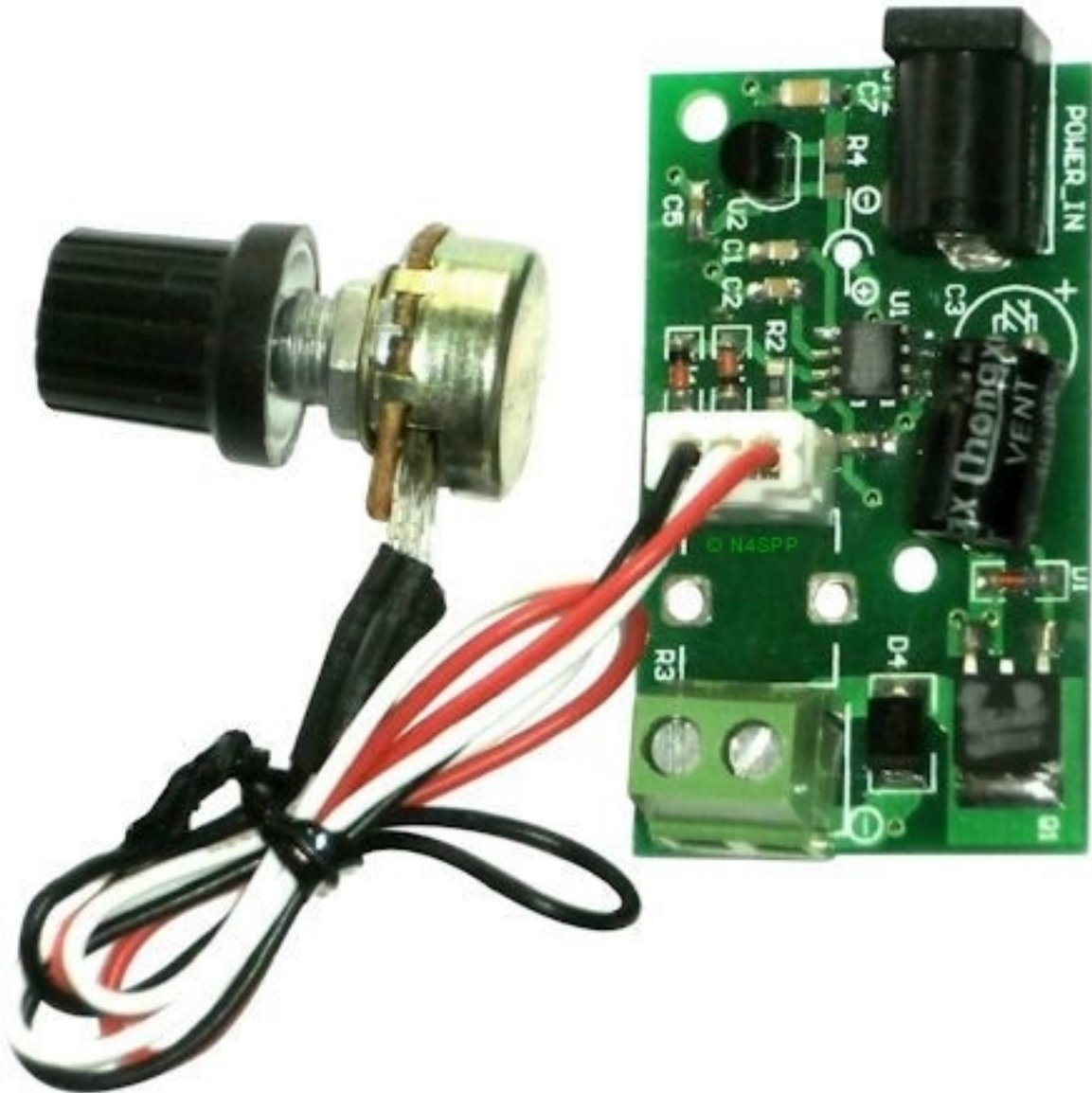
Figure 133: The small PWM speed controller card
