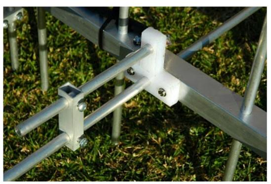
Above: Photo of the gamma match showing the teflon standoff. To the left of the top section of the teflon the braid connection can just be seen going to the boom and to the right the inner connection.
