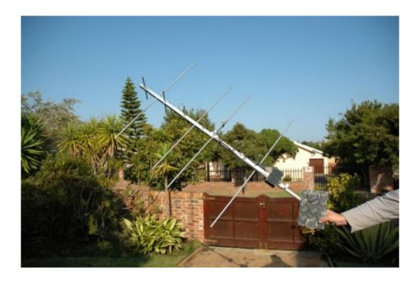
Above: "Bow and Arrow" Antenna of ZS2I. (NOTE: The plastic end caps must still be installed on the tips of the elements to complete the antenna. The plastic black box houses the homebrew diplexer.)
