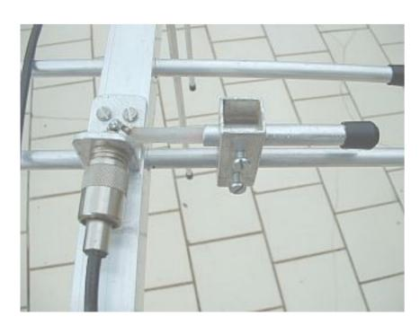
These dimensions and type of gamma match resulted in an SWR of 1:1 on 70CM's and 1.2:1 on 2M's on the center frequencies and 1:3 on 70CM's and 1.5:1 on 2M's in the band edges.
