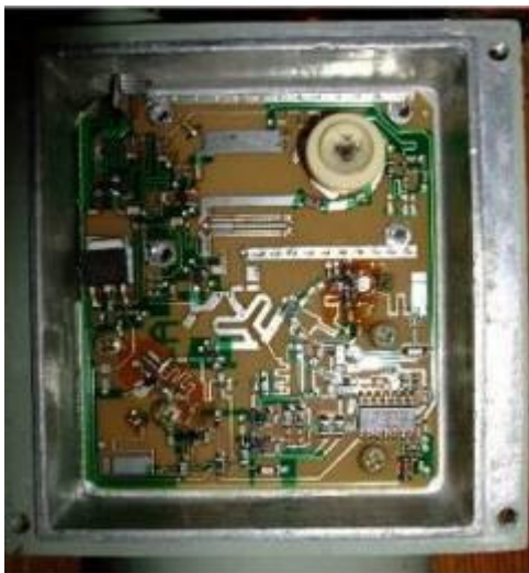
Figure 3: Unmodified C-Band LNB (DRO lid and housing removed)
