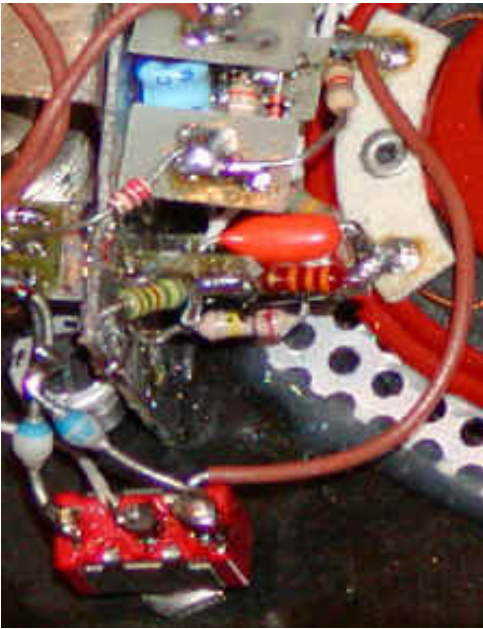
Figure 3: Close-up of diodes and the power switch
