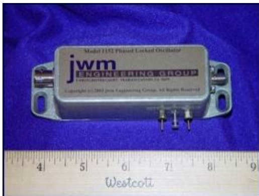
Figure 5: The 5170 MHz PLL LO with impressive +7dBm output
