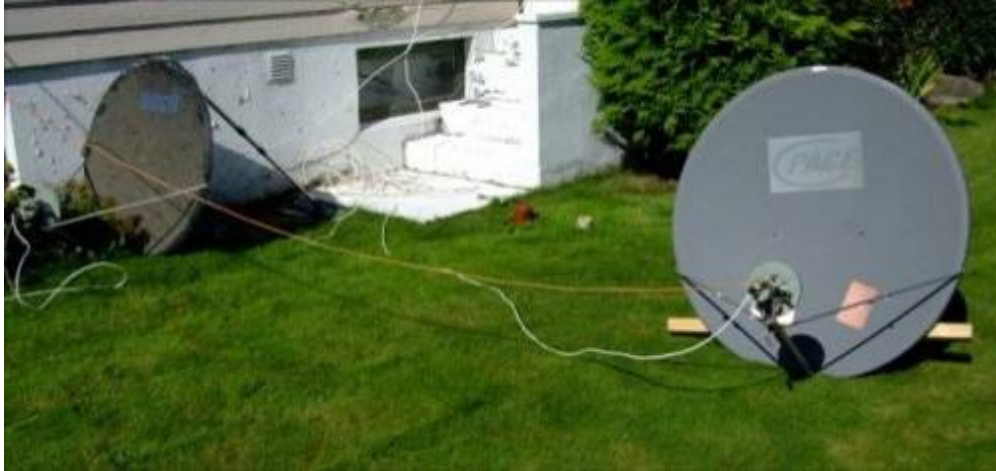
Figure 9: The two-dish (1 meter) interferometer (seen with common 5170 MHz LO feed)
