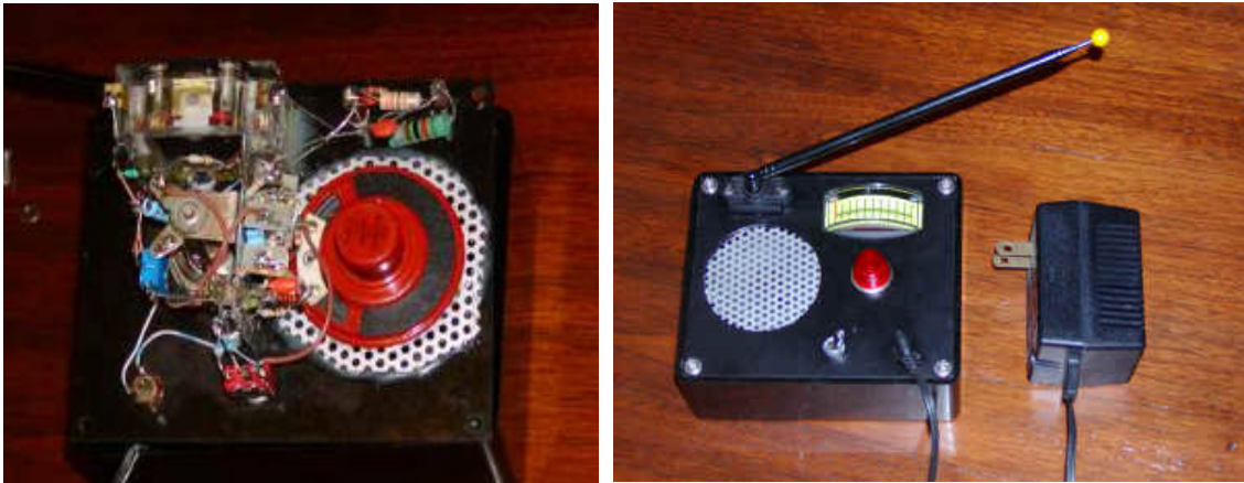
Figures 4 and 5: Prototype lightning detector with 5-volt lamp driver, meter circuit, and speaker circuit
