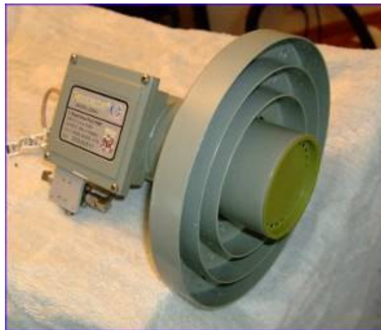
Figure 6: Ready to go C-band LNB unit
