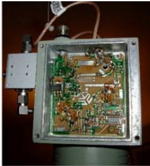
Figure 4: Modified LNB with outboard mixer
