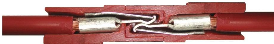
The above cut away view shows two Powerpole® housings connected to each other. This view shows how the contacts face each other and the locking tabs that are internal to the housings.
