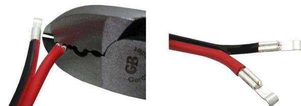
3. The housings have built-in interlocking tabs so you can connect them together. Interlock one red and one black housing as shown. Note how the ends of the housings are in the same direction as shown.
