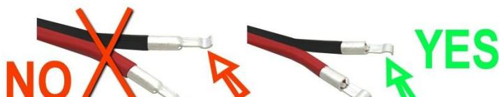
Note how the curved part of the contact is facing compared to the Red and Black wires
