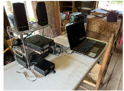
CW station setup at FD 2025 (FT-100D, FC-20 auto tuner, Ten-Tec 607 keyer paddle, amplified speakers and PC for logging). A new fan dipole antenna (designed and built by Conard, WV8JCR) worked like gang busters.
