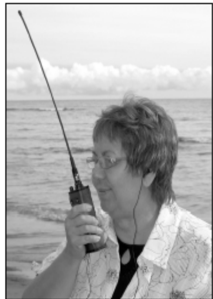
The author's wife, Kate Baker, KB10GF/VA30GF, makes a contact through the AO-51 satellite on the shores of Lake Huron in Michigan with her Kenwood TH-78A dual band HT. The extended "rubber duck" (MFJ Model 1717 from MFJ Enterprises) antenna and about 5 watts of uplink power provides just enough gain on the uplink and downlink to briefly work the satellite on near overhead passes.
