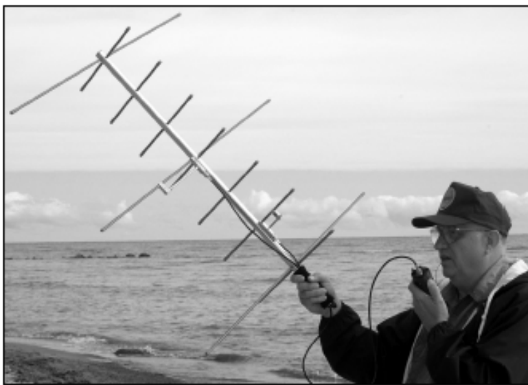
The author uses a Kenwood TH-78A dual-band HT and a lightweight Arrow Antenna to make a contact through AO-51 from the shores of Lake Huron in Michigan. When used with a 5 watt, full-duplex handheld in an open location free of foliage, such as a beach or a field, the antenna provides enough uplink and downlink gain to successfully work the FM birds, even on passes close to the horizon. (KB1OGF Photo)
