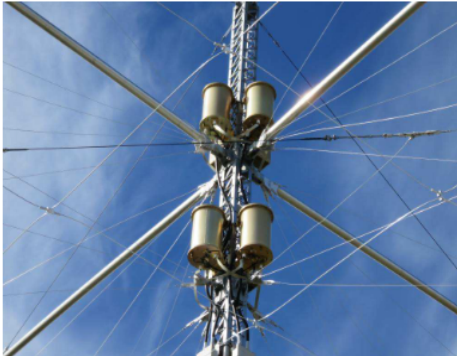
Figure 15 ~ Cylindrical antenna matching units, one for each upper and lower frequency crossed-dipole elements. Note the straps from the matching units to the dipole elements. The ground plane wires are closest to the camera and form a square pattern or mesh. Image © 2016 W. Reeve
