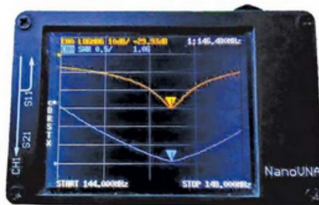
Figure 2 — My NanoVNA displays the return loss (labeled LOGMAG) as -29.93 dB, and the SWR as 1.06 to 1. The SWR scale is set for .5 units per division, and the LOGMAG as 10 dB per division. The default display of the NanoVNA is LOGMAG, the negative of return loss. You can select the SWR plot using the DISPLAY/FORMAT menu. The authors of the NanoVNA software must consider LOGMAG as the more useful type of display. Other instruments often default to SWR. The antenna being measured is my version of the "Stealth Rooftop Antenna" described in this issue.
