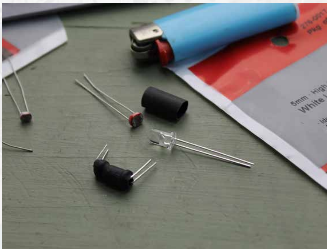
A homemade Optocoupler with only three simple parts.
