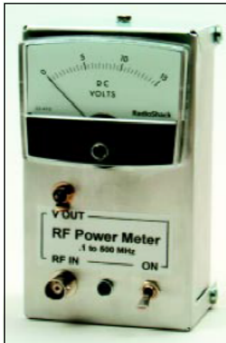
This version of the power meter is built in an inexpensive RadioShack utility box.
