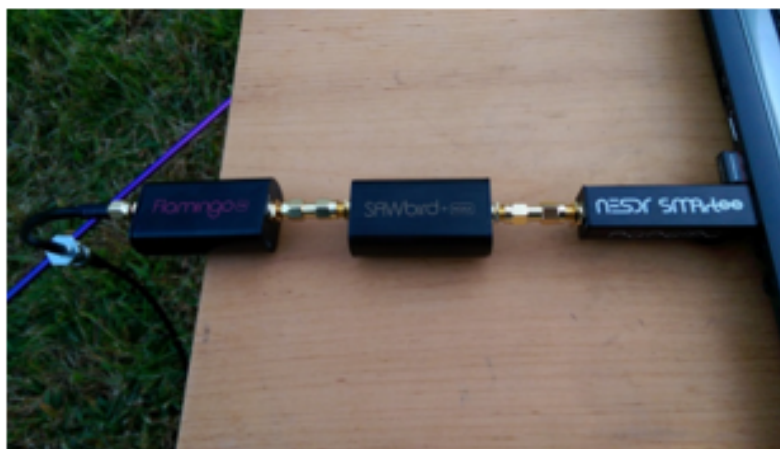
NooElec NESDrtee Dongle with a SAWbird LNA and broadcast FM filter
