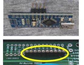
Now is the time when the choices you made for the NANO's sockets will come into play. If you chose to do the better (blue circled) arrangement, you should be able to use the conventional pin header for the DDS module, and install it either in the normal fashion as shown in the top photo at right, or spaced above the board as in the second photo. You can let the pins be just flush with the bottom surface of the board, which will elevate the header a mm or so.
