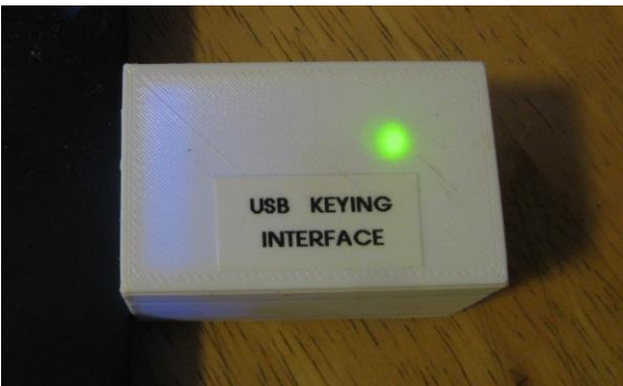
Completed optically isolated keying interface connected to PC's USB port. The SMD LED keying monitor is visible through a thinned out region of the 3D printed top cover.
