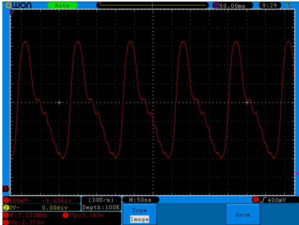
This next ‘scope trace shows the output of the power amplifier and low pass filter, taken across a 50 ohm resistive dummy load. The nice 38.6 Vpp sine wave allows a calculation of the output power as approximately 3.7 watts. Thus the gain of the final stage is about 17 dB! Power supply voltage, measured on the PCB, was 12.5 V, and total current draw was 630 mA (~ 50 mA for the TT2 portion) for about 50% efficiency of the PA.
