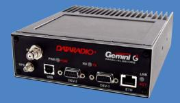
Capitalizing on over 20 years of experience designing mission critical wireless data equipment, Dataradio proudly presents the GeminiG3. This native IP mobile data modem operates at 128 kbps over 50 KHz channels at 700 MHz or 64 kbps in 25 kHz channels over 800 MHz and UHF channels using proven FM technology.
