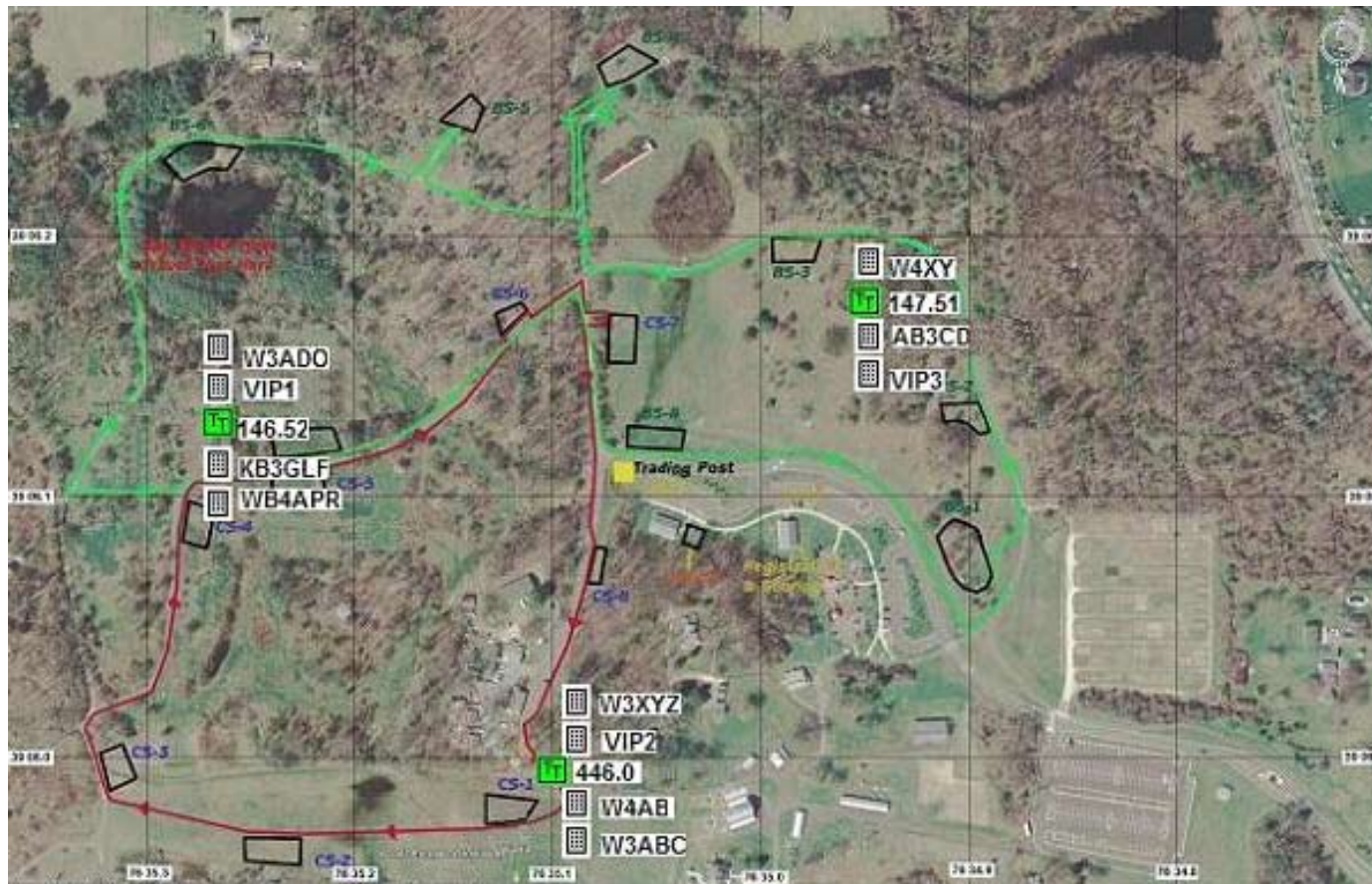
FIGURE 4. A TYPICAL EVENT MAP SHOWING HOW THOSE DTMF OR EVEN RFID USERS WOULD BE PLOTTED ON ALL APRS MAPS AT THE EVENT. THE DTMF USERS ARE SHOWN AS A LIST IN THE VICINITY OF THE FREQUENCY OBJECT ON WHICH THEY WERE HEARD. THE RFID USERS WOULD BE PLOTTED IN THE VICINITY OF THE RFID READER DEVICE THAT PICKED THEM UP.
