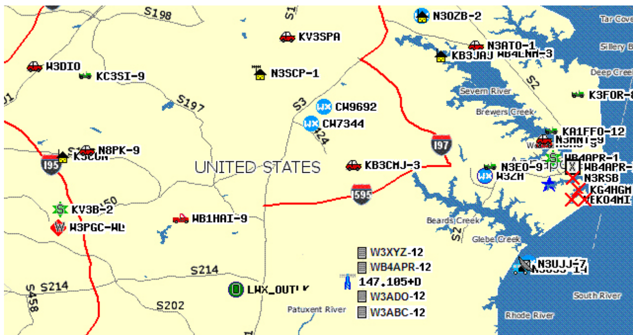
FIGURE 1. TYPICAL APRS MAP, BUT NOTICE THE DTMF OR RFID STATIONS IN THE LOWER RIGHT SHOWN AS BEING IN THE VICINITY OF THE 147.105 REPEATER.
