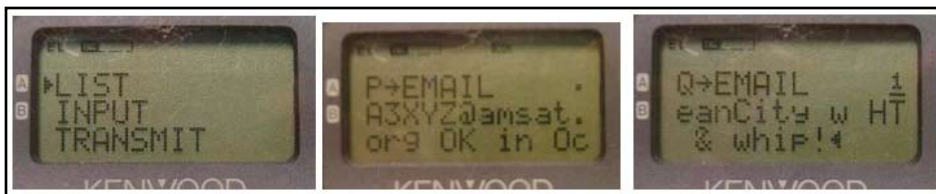
Figure 2. This shows the message menu and a typical APRS message. In this case, it is an e-mail to A3XYZ@AMSAT.ORG
