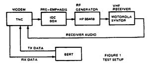
For these tests, the output of the TNC modem was connected through an IDC Box into the fm input of an HP 8640B signal generator. The IDC Box contains the pre-emphasis and clipping circuitry of a Motorola Motran transmitter. The used for these tests was a Motorola VHF Syntor. It had a 20 dBQ sensitivity of -121 dBm (0.2 uV).
