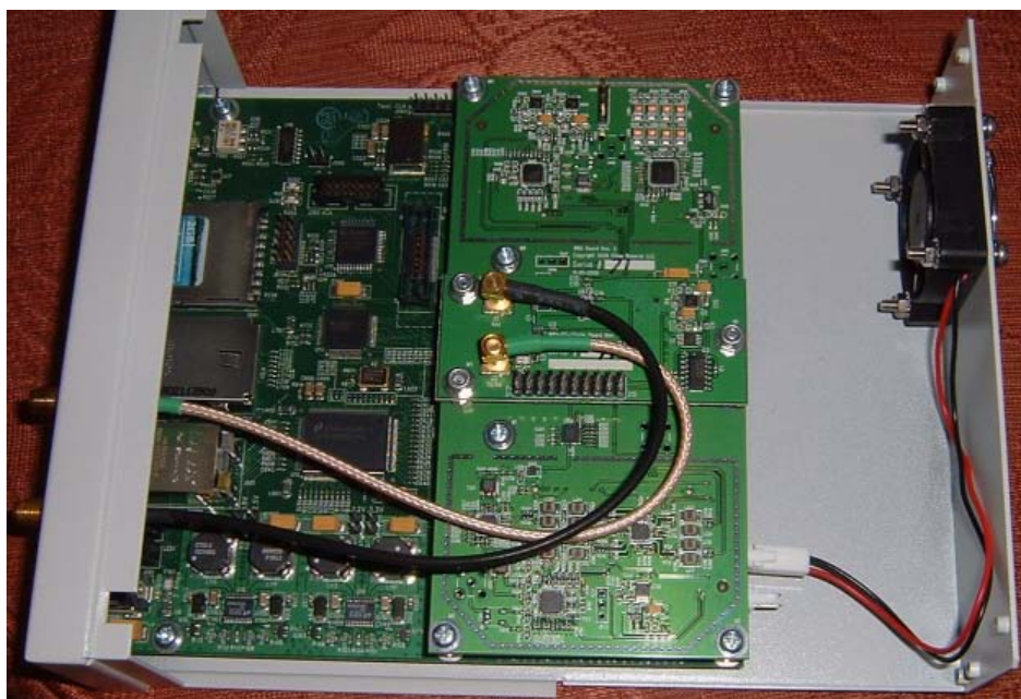
Figure 1. Inside the USRP2 with WBX board fitted.
