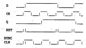
Next, the synchronized clock is applied to one input of EXCLUSIVE-OR gate 2, with the data applied to the other input. The output is Manchester encoded data suitable for JAS-1.
