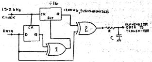
The TNC-provided clock of 19.2 kHz is 16 times the desired 1200 Hz clock signal. So, we apply the clock to a divide-by-16 counter and voilal we have our 1200 Hz clock.
