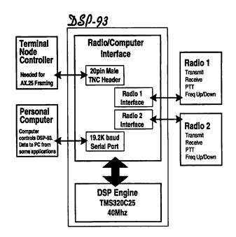
Interface Board, top board, contains two eight-pin female mini-DIN connectors for radio interfacing. Incoming radio signals pass through a voltage divider to establish the initial levels, then through an eight-channel multiplex chip. The multiplex chip then feeds the single A/D input with either of the two radio inputs or one of the six auxiliary inputs. The Texas Instruments TLC32044
