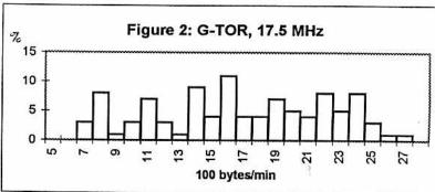
2099 and what appears to be a peak at the speed of 1500 to 1599 bytes per minute. This graph shows all the data speed results from the 145 separate test runs which were made in the same time interval as those shown in Figure Three for the Pactor mode.
