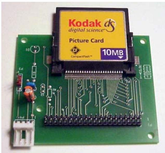
Figure 2: The TAPR CompactFlash Adapter Card, with a 10-Mbyte Kodak CompactFlash card. The adapter card turns the CompactFlash card into a 100% IDE compatible solid-state hard disk, able to operate from -25(C to +75(C, perfect for those cold mountaintops and hot deserts.
