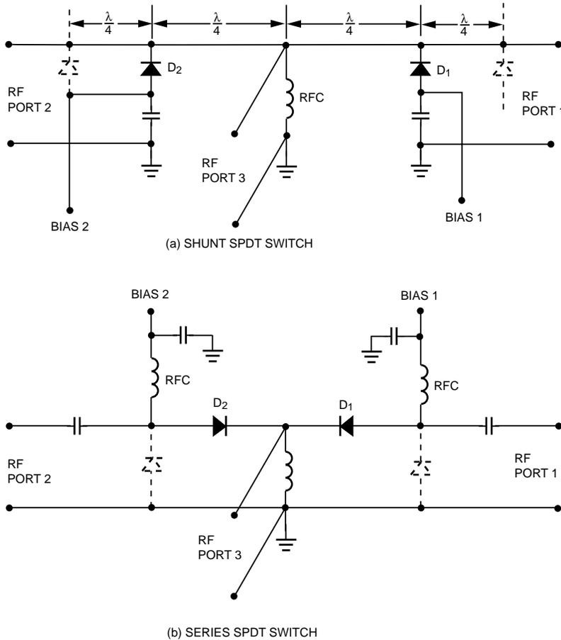
Figure 15. Multiple Throw PIN Switches.
