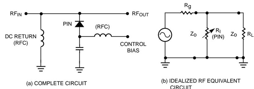
Figure 8. Shunt PIN RF Attenuator or Switch.
