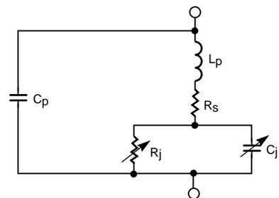
Figure 2(a). PIN Low Frequency Equivalent Circuit.
