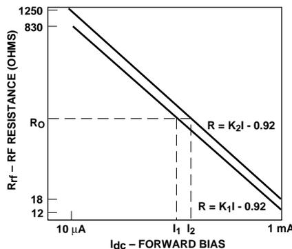
Figure 4. Matching of PIN Diodes by Offset Current.
