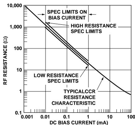
Figure 3. Typical RF Resistance versus Bias Current for HPND-4165.
