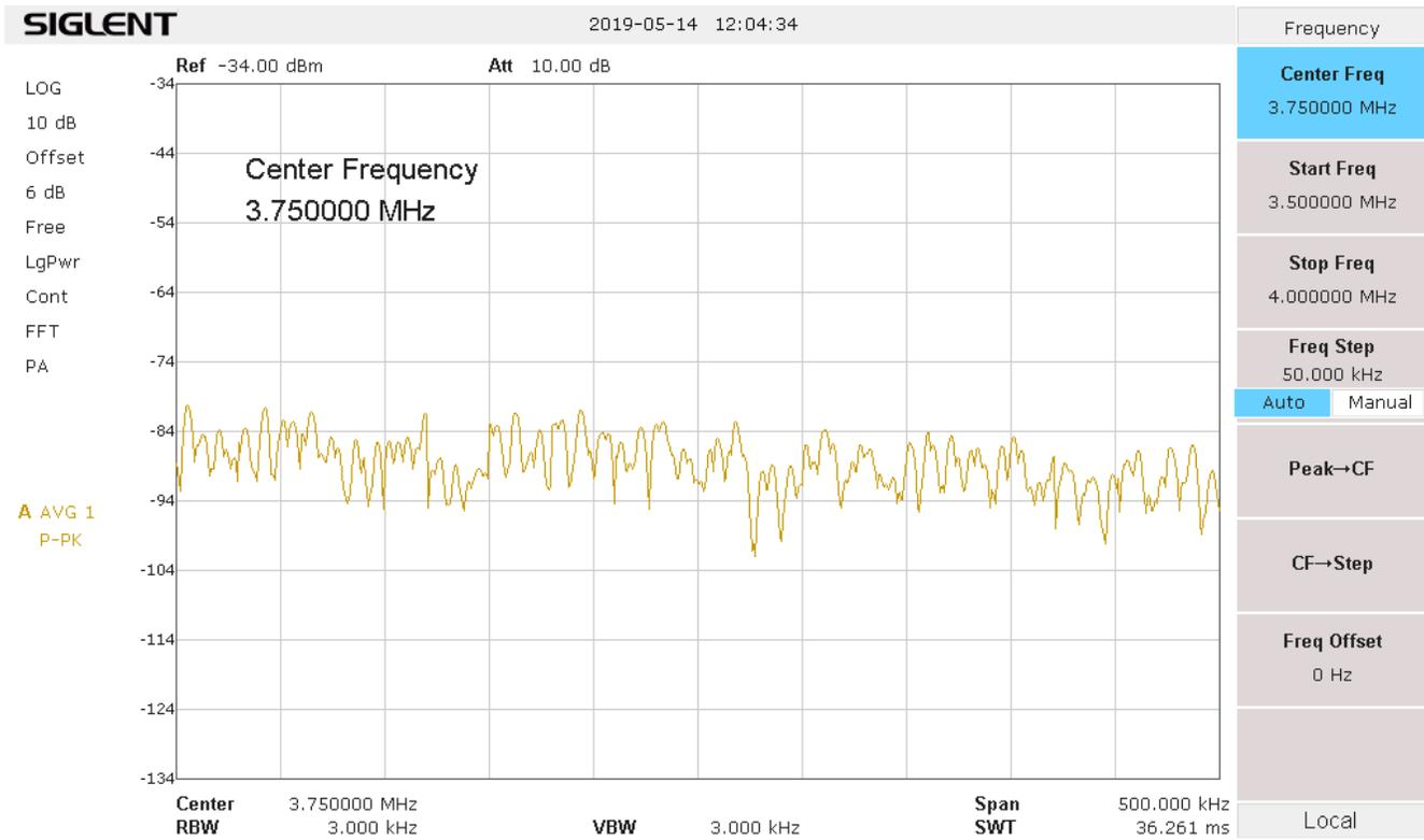
The 3.5-4 MHz plot above shows noise in the range of -84 to -94 dBM (3 kHz bandwidth).
