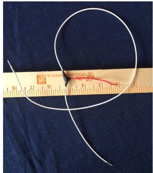
4. **We want TWO turns** (remember, one passage through the interior of the toroid is a "turn") created out of the 7" section of the white wire. Set the solder connection on the **OUTSIDE** of the toroid, and carefully wind two turns to one side of the solder joint. Pass the white wire through a zip tie and secure it.
