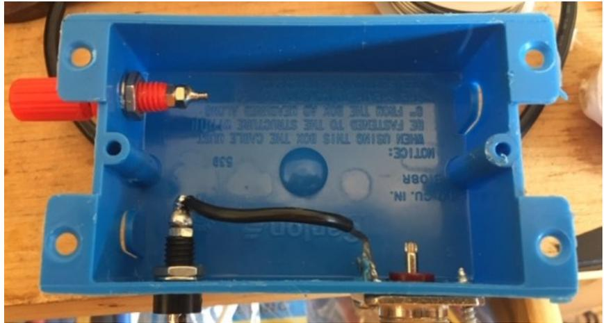
7. **Now make your solder connections from the Toroid.** The longer end of the white wire goes to red banana plug. The shorter side of the white wire solders to the ground wire from the SO-239. The Red wire solders to the center connection of the SO-239.
