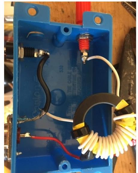
8. Wrap the soldered connections with **electrical tape** to avoid unwanted shorts
