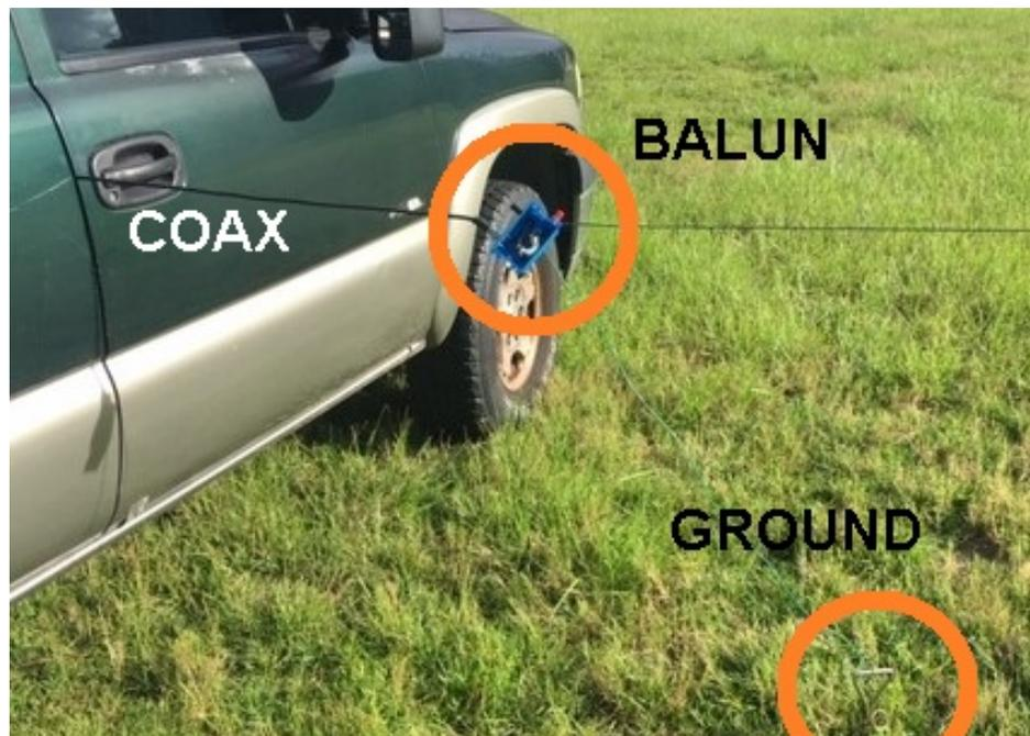
With the Antenna being 135 feet of #14 stranded wire pulled up into an oak tree. I was surprised at how much tension was required to try and elevate this--- you may want to put a small loop in the wire (won't add too much inductance) and use another small rope to tension it, as you do not want a lot of tension on the banana plug jack.
