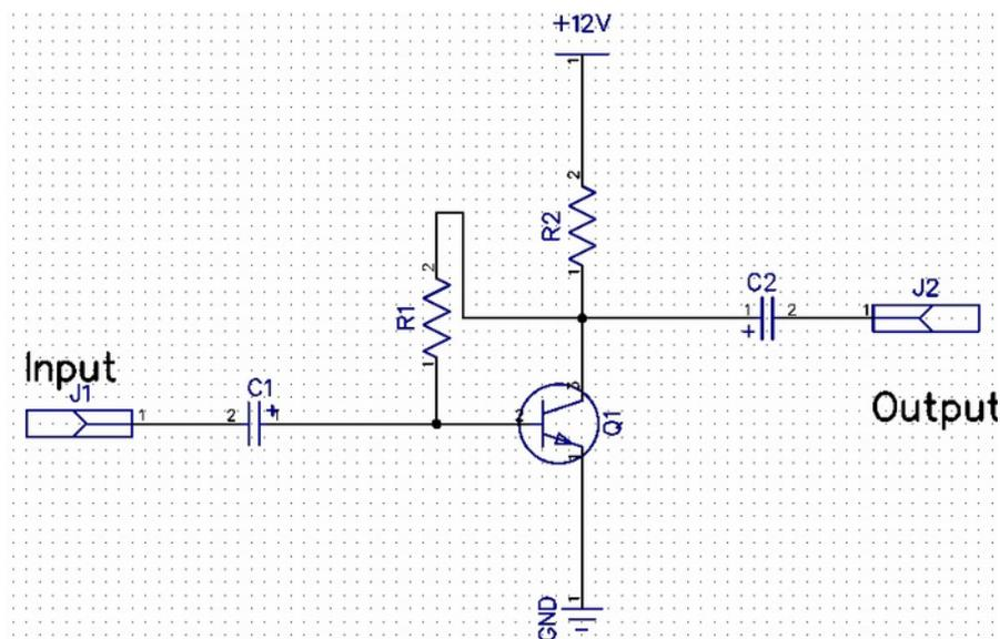
An easier to adjust biasing scheme is to get the biasing voltage for the base pull-up resistor R1 not from the positive supply....but from the COLLECTOR!!
