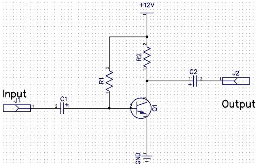
The very simplest biasing is simply to connect a resistor from the positive supply (assuming an NPN transistor like the 2N3904) to the base. A capacitor (C1) can be used to prevent the input AC signal source from “seeing” this voltage. A resistor in the collector circuit (R2) will cause a voltage gain to manifest, and another capacitor (C2) can be used so the output signal doesn’t have any DC to it.
