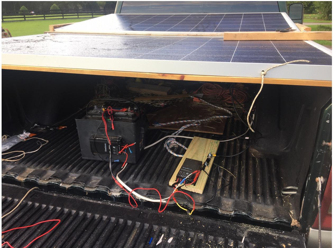
2 Solar Panels Secured to Pickup Truck, combined power approx 500 watts. However our MPPT controllers were only able to take advantage of approximately half that power due to temperature limitations. This could be improved with larger MPPT controllers.
