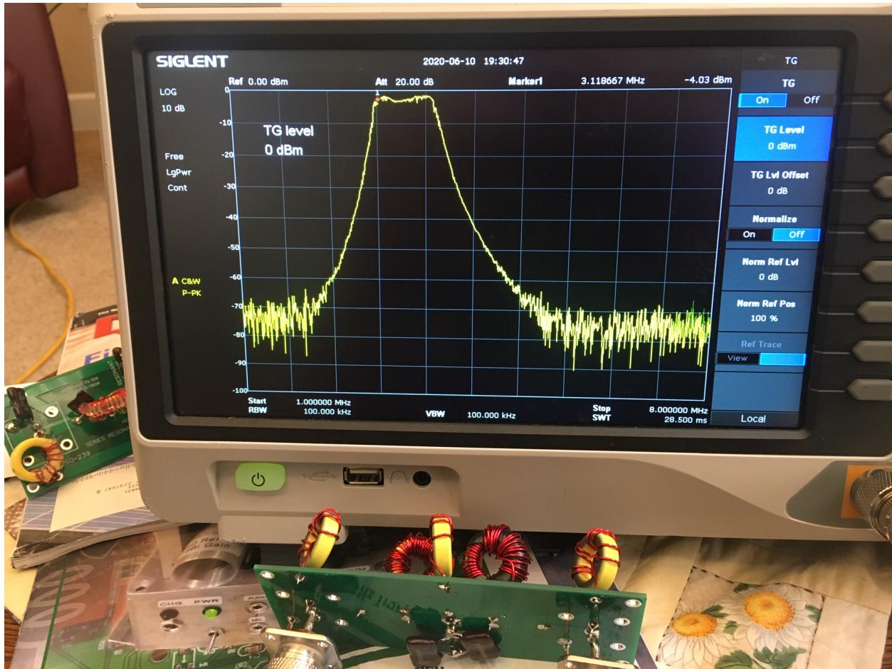
Magnificent 80 meter band pass designed by John Trites N05X
