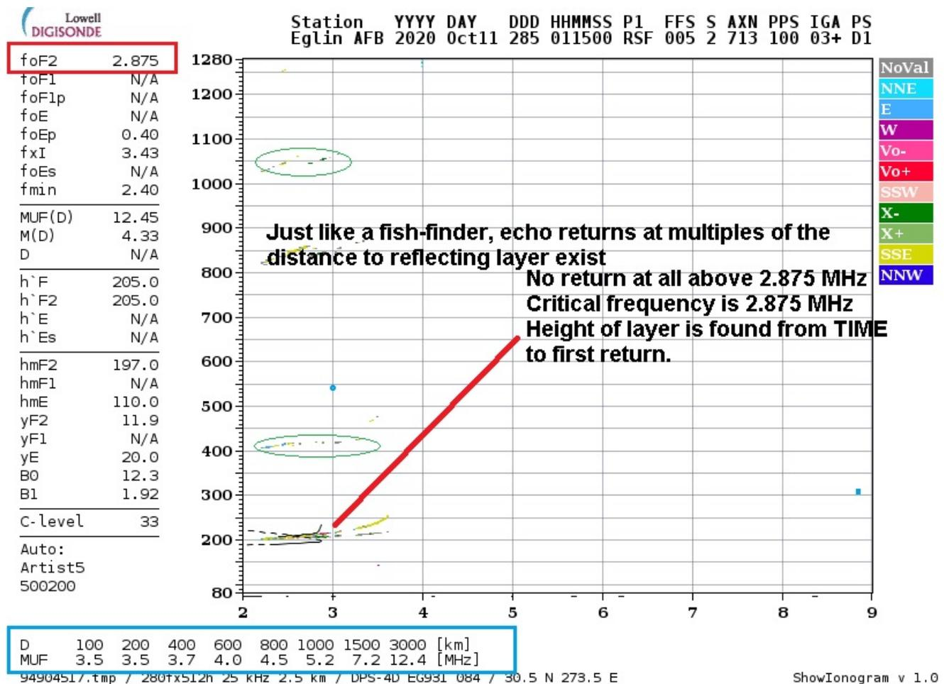
**Red Box:** foF2 = critical frequency for the F2 ionospheric layer
