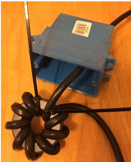
4. Stuff the wound toroid into the plastic outlet box and secure with the gray cover.
