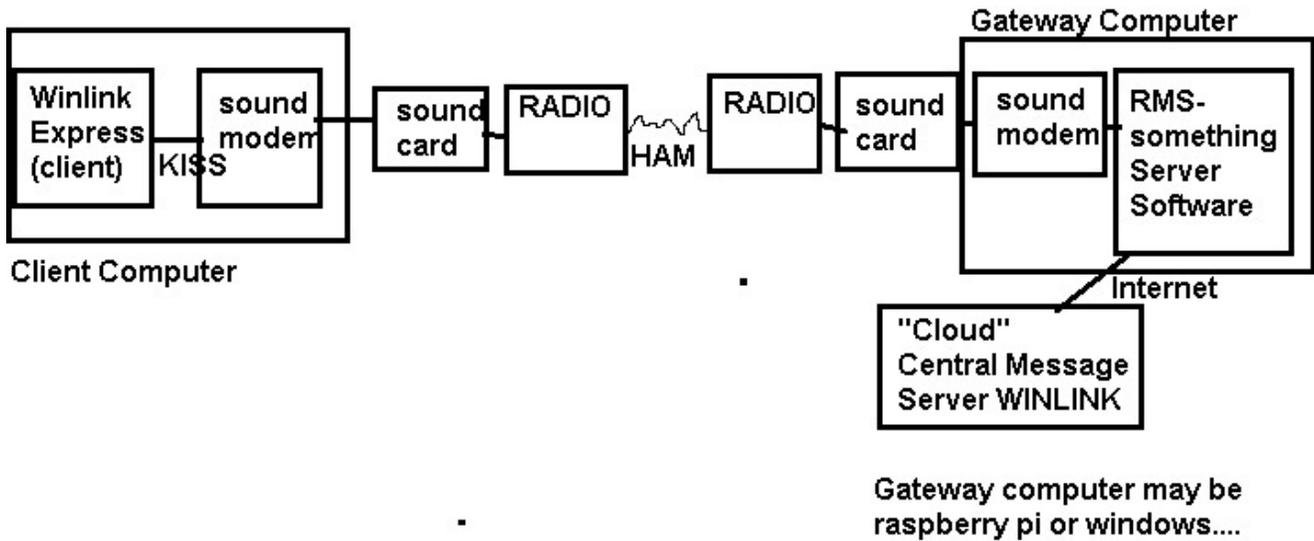
Figure.6 Winlink client typically sends KISS-framed messages to port 8100 of the same computer where soundmodem picks them up and gets them going out to the radio, over the ether, and back again to the RMS server software which receives them as KISS framed messages from its version of soundmodem, whatever that is for whatever operating system the server is operating.
