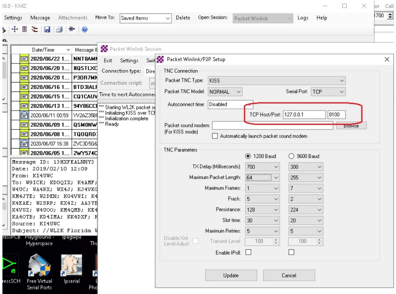
Figure9 . Note the TCP Host is the LOCAL computer (special ip number 127.0.0.1) and port 8100 so that it links up to soundmodem. You can use any of a number of ports (as long as they aren't already in use!) if both programs are expecting the same number. The other settings for TNC Parameters are for a very modest performance radio....
