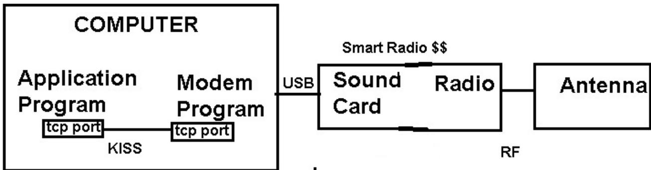
Figure 4: *Moving the sound card inside the radio made a new product, the smart radio.*
