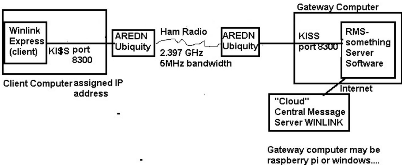
Figure 7. Replacing the winlink vhf connection with a microwave ham radio connection
