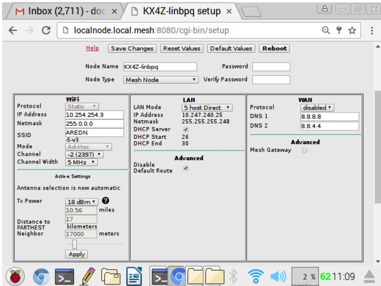
Figure 13. This is ONE of the various setup pages on a AREDN mesh node web-based controller. Note at the lower left you can set the TRANSMITTER power – I have it throttled back to 18dBm here....(63 milliwatts)
