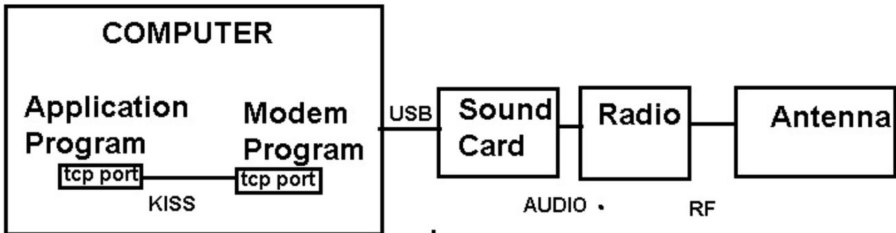
Figure Three: *With the advent of cheap soundcards, even more of the smarts got cheaper and became free modem program software like “soundmodem.exe”*
