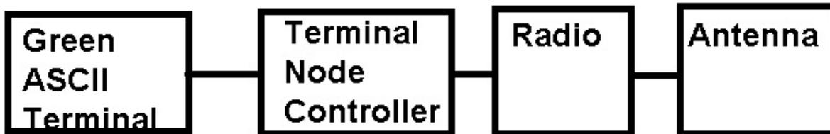
Figure 1: *How amateur radio operators send digital characters back 45 years ago.*
