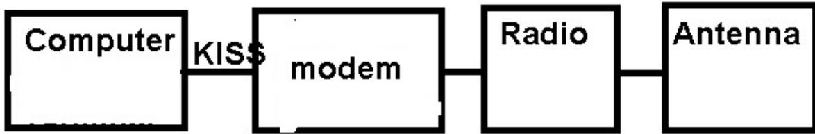
Figure Two: *More of the smarts moves into the computer; communications with the hardware modem are by KISS*
