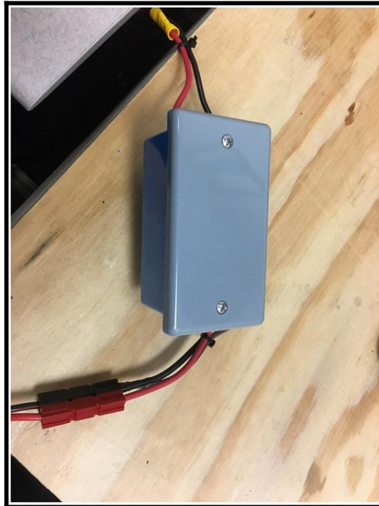
*Polarity Protector added to EOC existing transceiver.*
