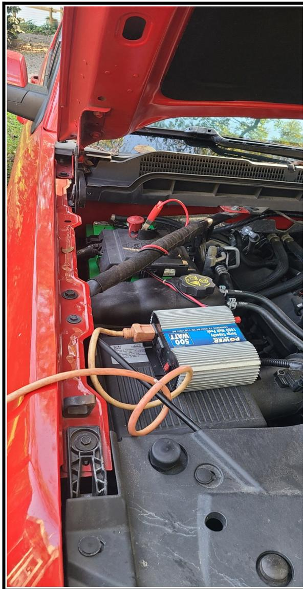
*Inverter positioned on vehicle battery, with extension cord to radio equipment*
