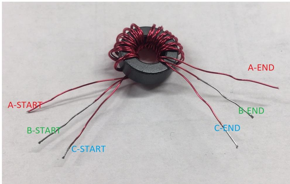
Now comes the important part. We're going to tie the C (start) winding to the B (end) winding so that we have the B and C connected in the proper phasing and we end up with nice center tapped winding.
