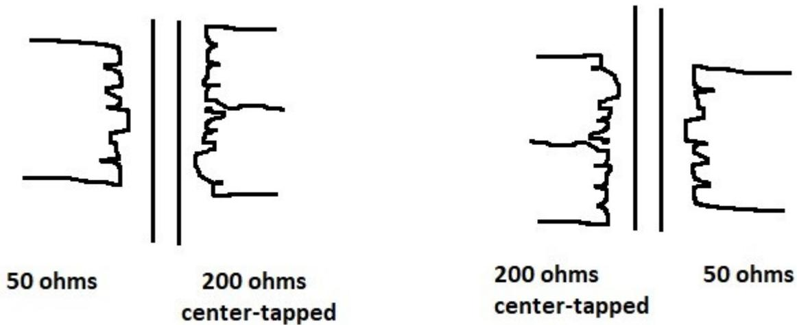
The lower-impedance side has 10-13 turns and the higher-impedance side has 20-26 turns, depending on how many “fit” on your toroid.
