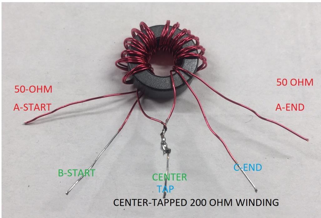
We can now use this type of transformer as either a step-up (with a center tapped secondary) or a step-down (with a center tapped primary) impedance transformer. See the drawings below:
