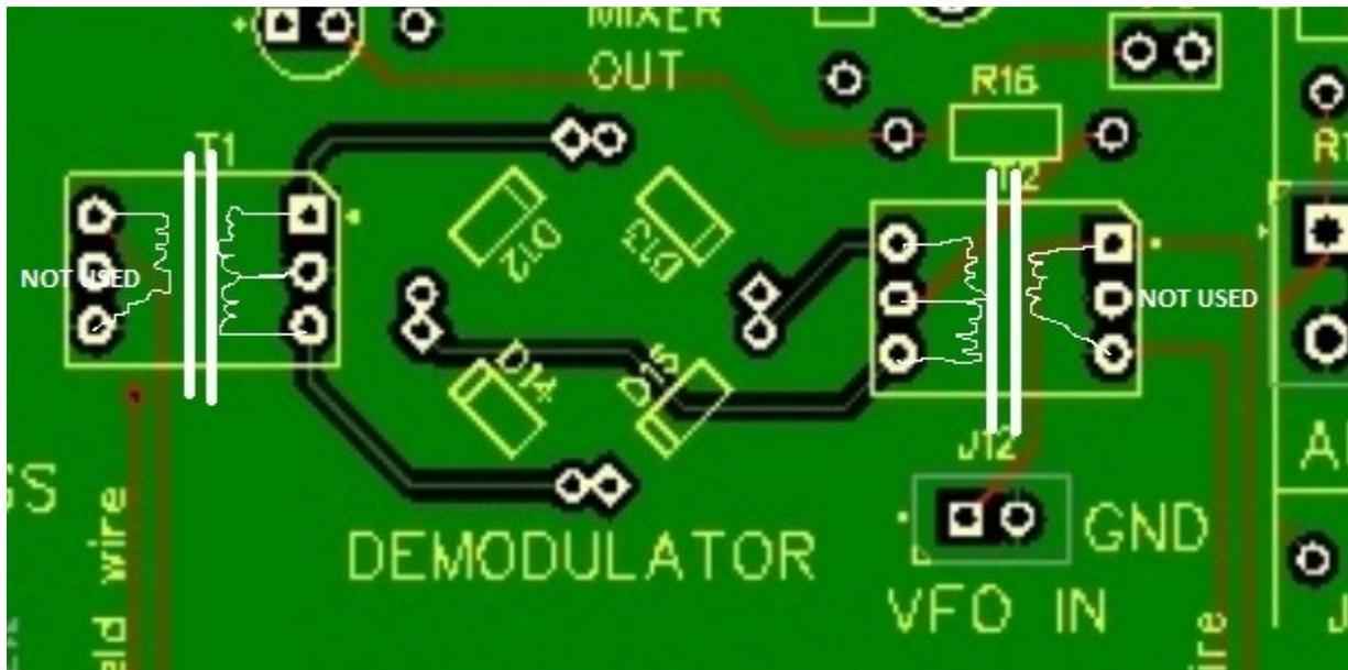
Note that the center-tapped high impedance winding side goes closest to the demodulator diodes on both sides. The lower-impedance (non center tapped) side goes to the OUTSIDE away from the demodulator diodes. The middle solder pad on the lower impedance (outside) side is not used.
