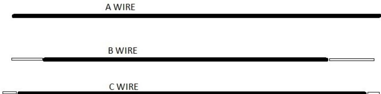
Then using either simple manual twirling or a slow-turning electric drill, we twirl the three wires into a cord, with about 6-8 turns per inch.
