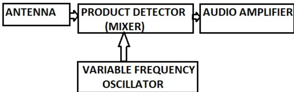
In this receiver, the audio amplifier is broken into two sections, a "preamplifier" and a "power amplifier." Our design is based on the DC40 direct conversion receiver (see <https://miscdotgeek.com/building-direct-conversion-receiver-part-1/> and <https://web.archive.org/web/20171109081542/http://www.phonestack.com/farhan/dc40.html> )/
