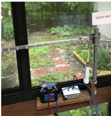
Yagyi Bullet Node Battery Powered
