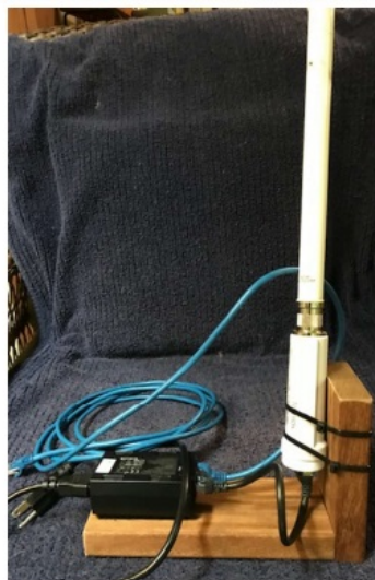
Omni Bullet Node AC Powered POE
