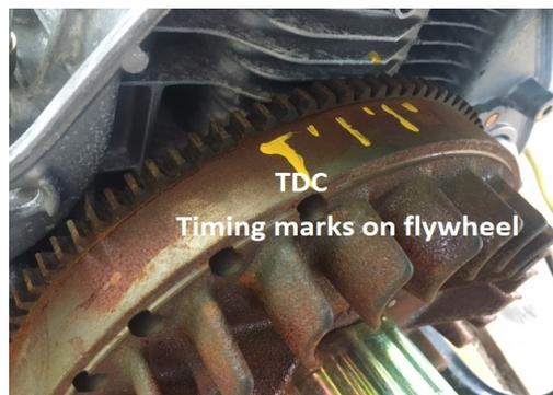
Off came the recoil starter, and housing, and I found the all important timing stamps on the flywheel/forced air fan. A bit of plastic insulation made a "straw" in the fuel pump outlet so I could try to observe the onset of fuel delivery (which continues for several degrees of rotation). It was WAY WAY too early. (4 degrees is a lot in diesel engines). I needed to delay another 12 degrees or so.
