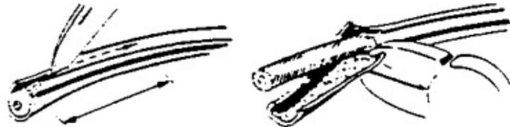
TWIST THE SHIELD WIRES INTO ONE STRAND. REMOVE THE INNER INSULATION. THEN APPLY A SMALL AMOUNT OF SOLDER TO THE END OF THE INNER LEAD AND THE SHIELD.
