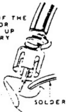
Newer commercial plugs (often with a screw on barrel) are much easier to solder together than the cheap simple connectors Heathkit had in their kits!
