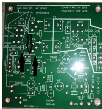
6. Finally, solder in transformers T1 and T2. They are symmetrical so can go either way.
