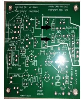
3. Solder in a "reed relay" to operate your radio's PTT circuitry. The relay's pins are symmetrical so up or down doesn't matter.
