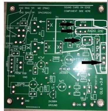
2. Solder a 1 or 2 or similar electrolytic microphone DC bias blocking capacitor. Note the + marking to the RIGHT. Many radios have +8VDC on the mic and the transformer would short this out without this capacitor.
