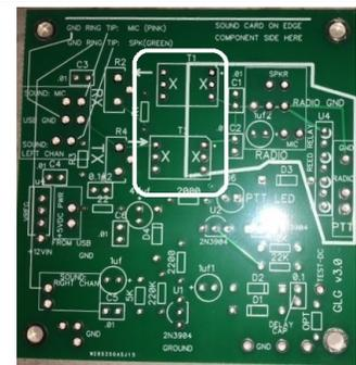
7. Solder four thin, flexible wires that will make the ground, mic, Left and Right channel output audio connections to the SOUND CARD.
