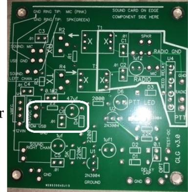
We don't normally use the 12V Regulator pads unless you're powering this board from a separate 12VDC power supply.
