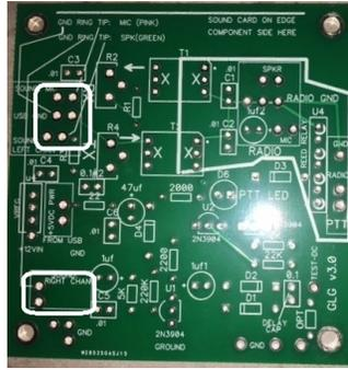
8. You may need help to solder the wires to the proper terminals on the Mic and Spkr jacks of the sound card. These have to be done quickly to avoid melting the jacks. Writing on the board shows you where to solder.
