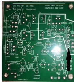
4. Solder in R2 trimmer potentiometer 500 ohms to set the signal level from the receiver to the sound card. Also R1, typically 4700-10,000 ohms to step down the received signal.
