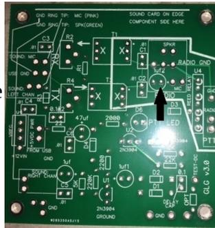
3. Solder in 0.01microfarad (uf) ceramic capacitors for bypassing unwanted radio frequencies at C1 and C2. (.001 will also work) If you later still have RFI problems, you can add two more at C3 and C4.
