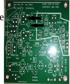
5. For the TRANSMIT signal level control, solder in R3 (typically 4700 ohms). For VHF solder in a 500 ohm trimmer at R4. For HF you may wish to run three wires out to a potentiometer to allow frequent adjustment. Capacitor "0.1#2" provides DC isolation in case your sound card has a DC bias.... C3 and C4 are optionally added if you have RFI problems.
