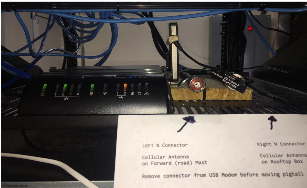
**Figure 2-8B:** *Mike Sprenger rigged up a rubberband system to keep the cellular antenna connected and made the system work far better!! This also tends to better physically support the USB connected 730L modem. Note which connector goes to which antenna. I’m not convinced that the “Cellular antenna on Rooftop Box” is useful.....*
