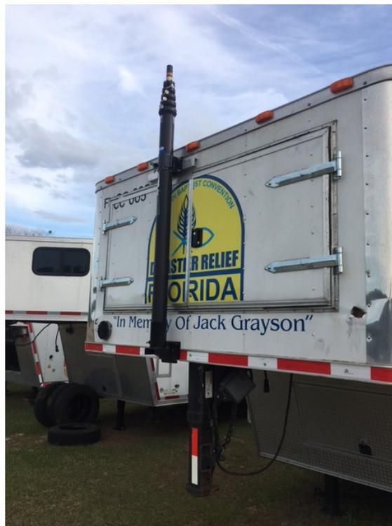
**Figure 2-18.** *Hurry Up Mast can be transported attached to the trailer and ready for deployment. Be certain that it is fully collapsed before travel however. It should be LOWER than the height of the AC systems.*
