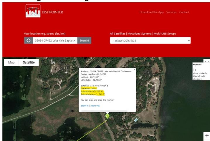
Figure 4-6 dishpointer.com delivery of aiming data
