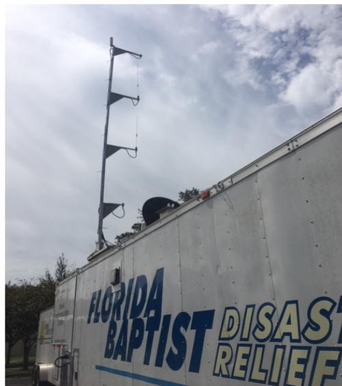
Figure 2-13 Roof mounted mast
