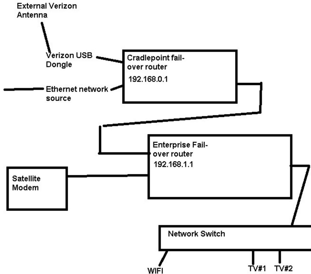
**Figure 2-6** *Block diagram of networking*
