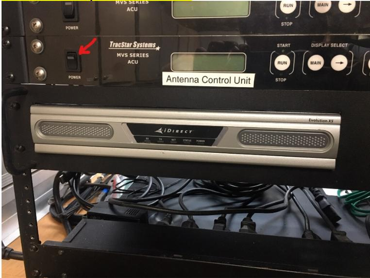
Figure 4-1 Antenna control Unit.
