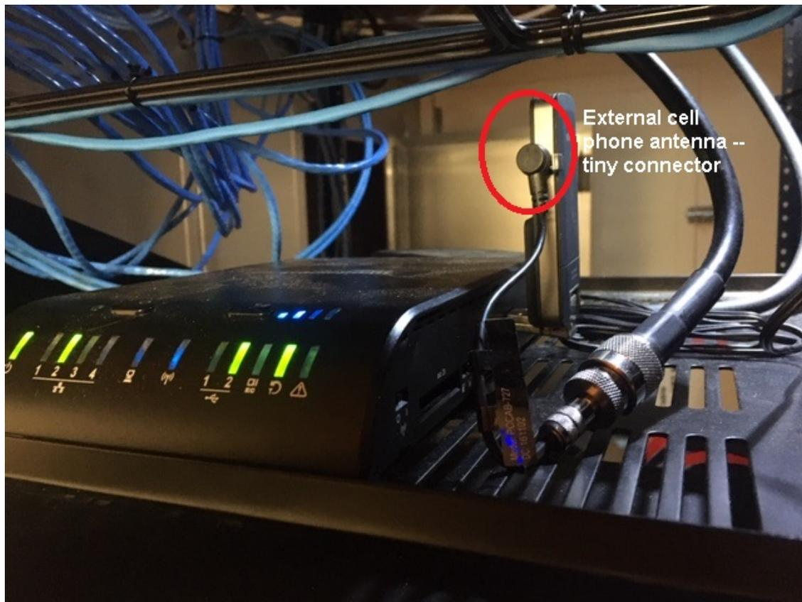
**Figure 2-9.** Red Circle shows the fragile connection of the external antenna to the Verizon hotspot, a USB input to the Cradlepoint fail over router. As shown in previous photo, Mike Sprenger has jury-rigged this with a rubberband, much more successful. In this example, the wired Ethernet has failed, and the system is preferentially routing Verizon data connection (from USB slot #2, note green light) onward to the Enterprise fail-over router.
