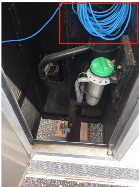
**Figure 2-7A** *PREVIOUS Storage of external wired Ethernet connections* **December 2020:** *Note that a female RJ-45 jack has been added to the left front edge of the trailer to allow external wired Ethernet to be easily connected. The wiring of this connector is the more-common “B” version of the EIA standard.*
