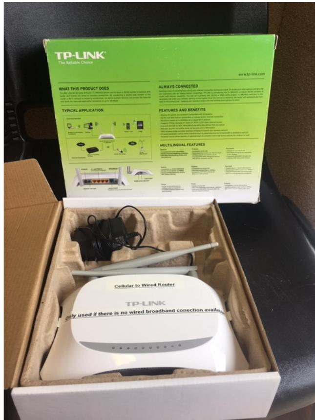
Figure 2-11 TPLink fail-over cellular/wired/wifi router
