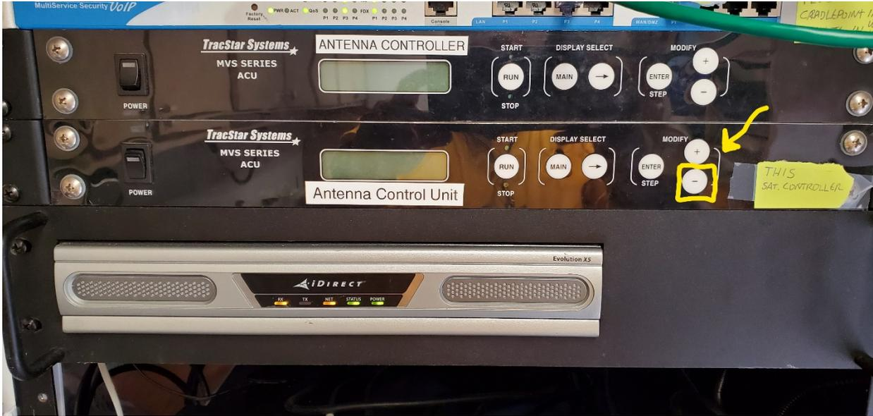
Figure 4-7 – the minus button used to begin the stowing process.
