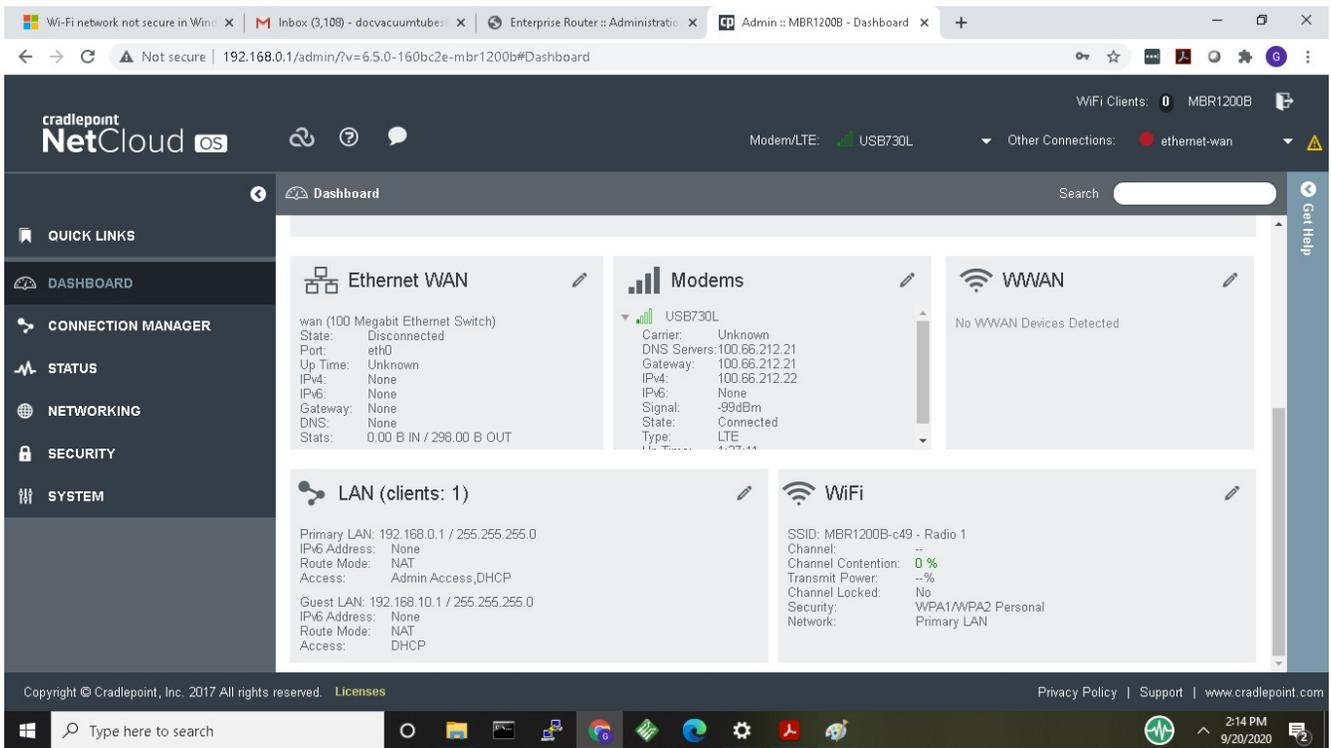
**Figure 2-8A.** The web server on the Cradlepoint allows you to see which connections are up and running, as well as the signal strength found on the Verizon Modem USB730L. The manual for the 730L is stored on the main ham computer in the directory [c:\Ham](#).
