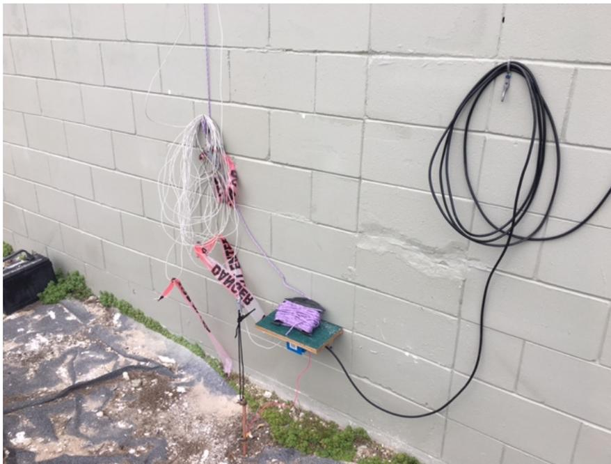
**Figure 2-16B:** *Staged End-Fed Antenna and balun at end of Warehouse. Antenna can be deployed by laying out toward the palm tree, connecting to cord there, and pulling tight. Coax runs to the typical parking position of the PCC Trailer.*
