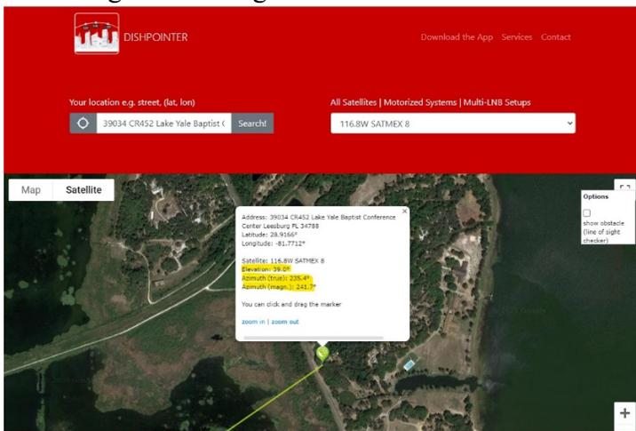
Figure 4-6 dishpointer.com delivery of aiming data
