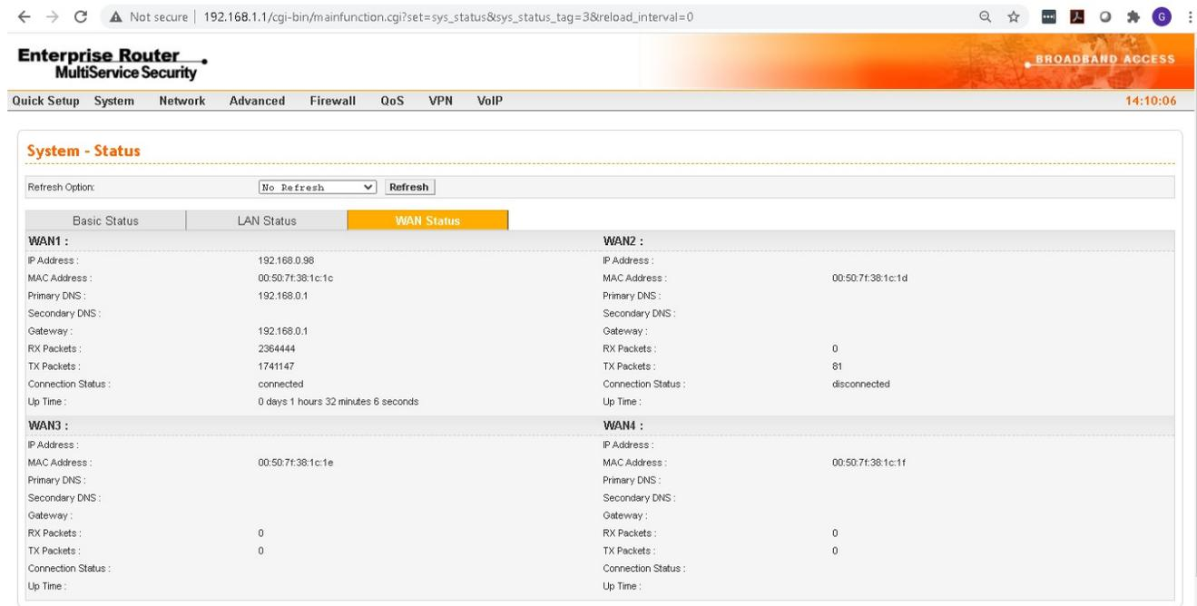
**Figure 2-10:** System status screen from Enterprise Router showing one working WAN connection; for this screen shot, the satellite signal was removed, so the screen displays only ONE working WAN connection.
