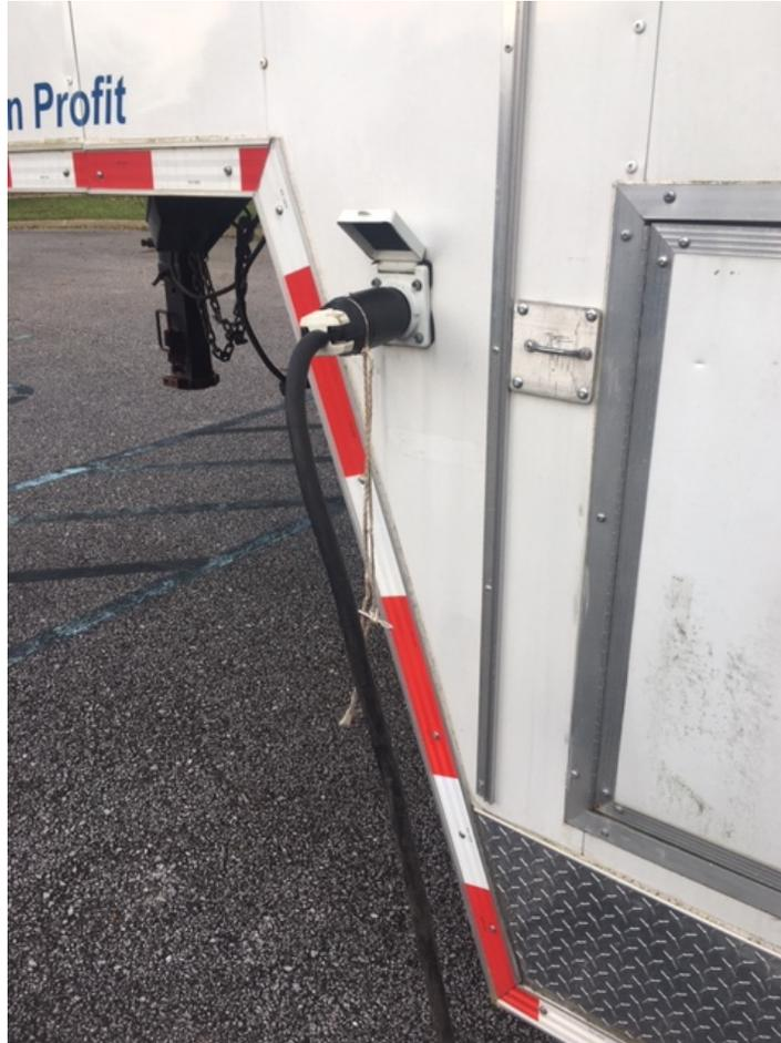
Figure 2-1 AC power connection.
