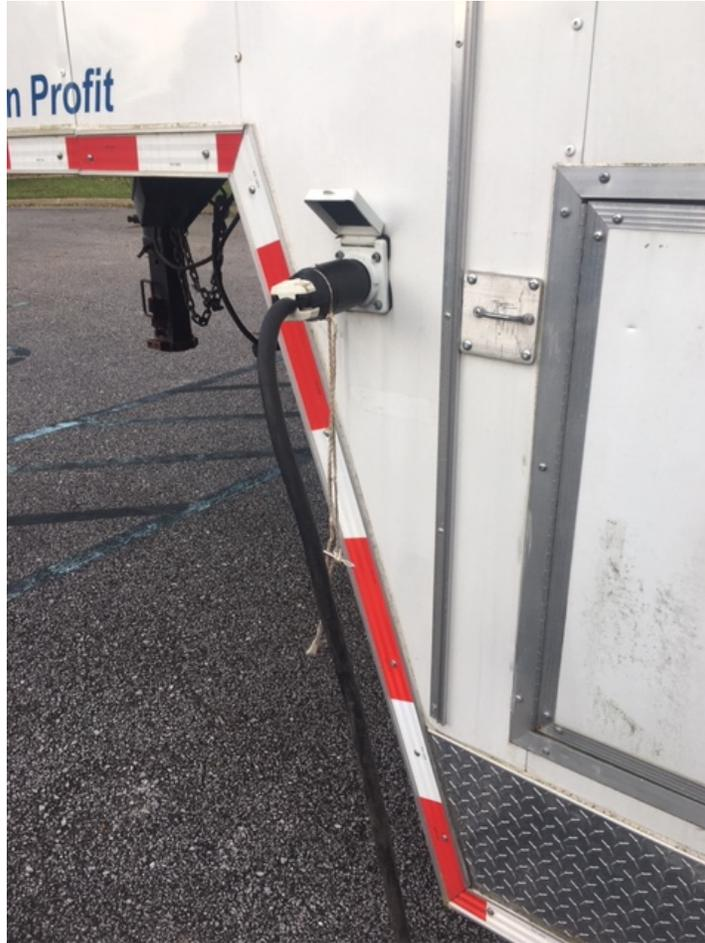
Figure 2-1 AC power connection.
