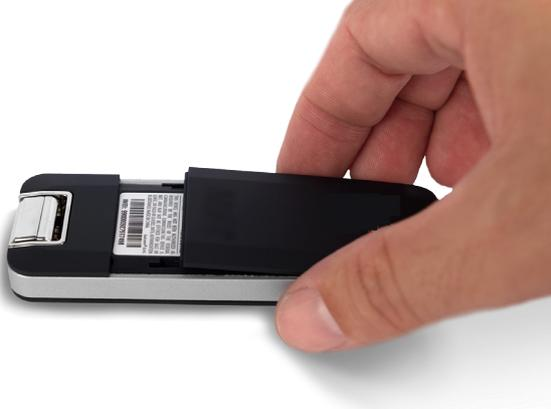
Insert the SIM Card with the contact points (typically gold-colored) facing toward the USB modem. Position the card with the notched corner as circled below and slide the card into the SIM slot.
