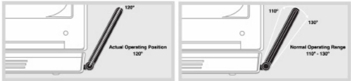
Please ensure that the modem is positioned as indicated in the illustrations to maintain SAR compliance and for proper performance. This modem has been designed and tested to meet SAR compliance as outlined by the FCC. If the modem is connected to USB ports other than those shown above please ensure the device maintains a separation distance of at least 5 mm.
