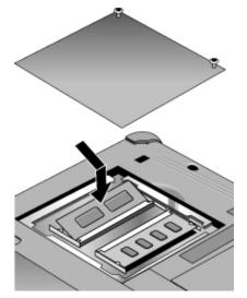
4. Insert the RAM expansion module into the connector at about a 30° angle until it's fully inserted. Then press down at both sides of the module until it latches.
