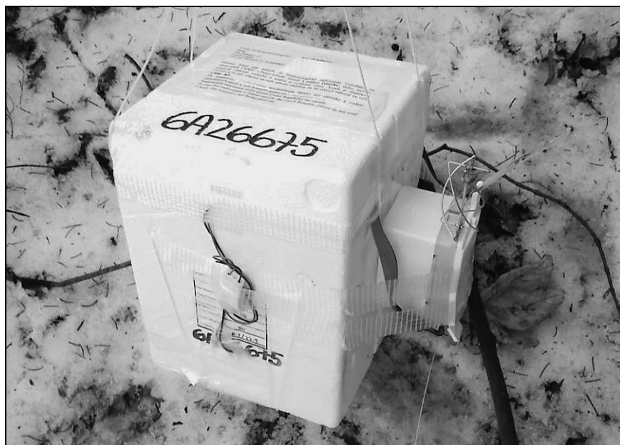
Nowadays sonde launched from the Czech Hydrometeorological Institute in Prague - Libuš, used for ozone measuring.
