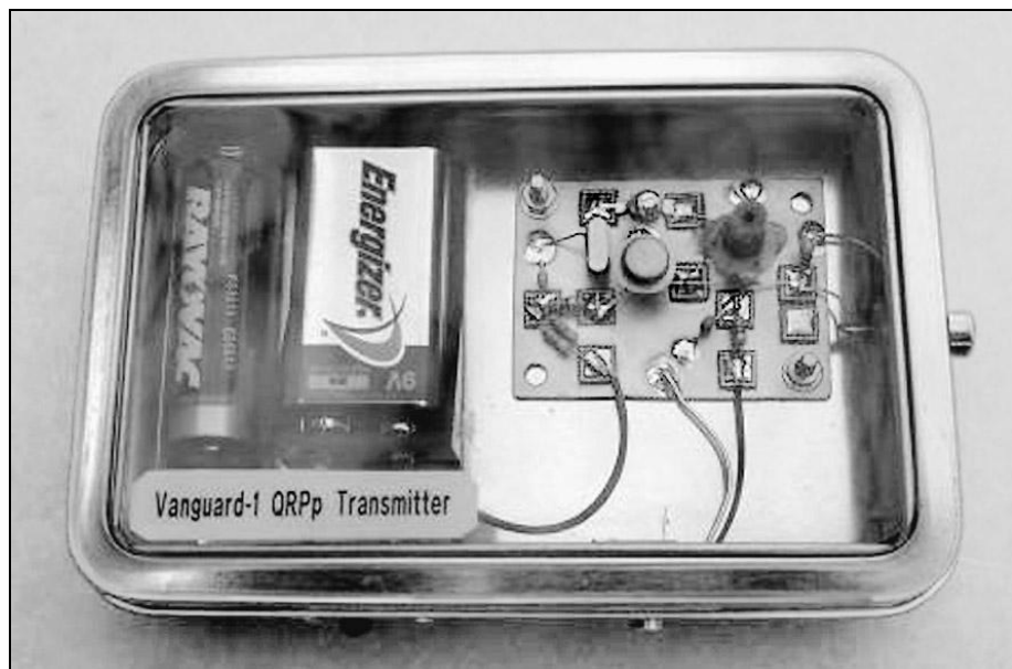
Carlo, IZ4KBS - 35 mW TX (GT313V, Ge-pnp), dipole
