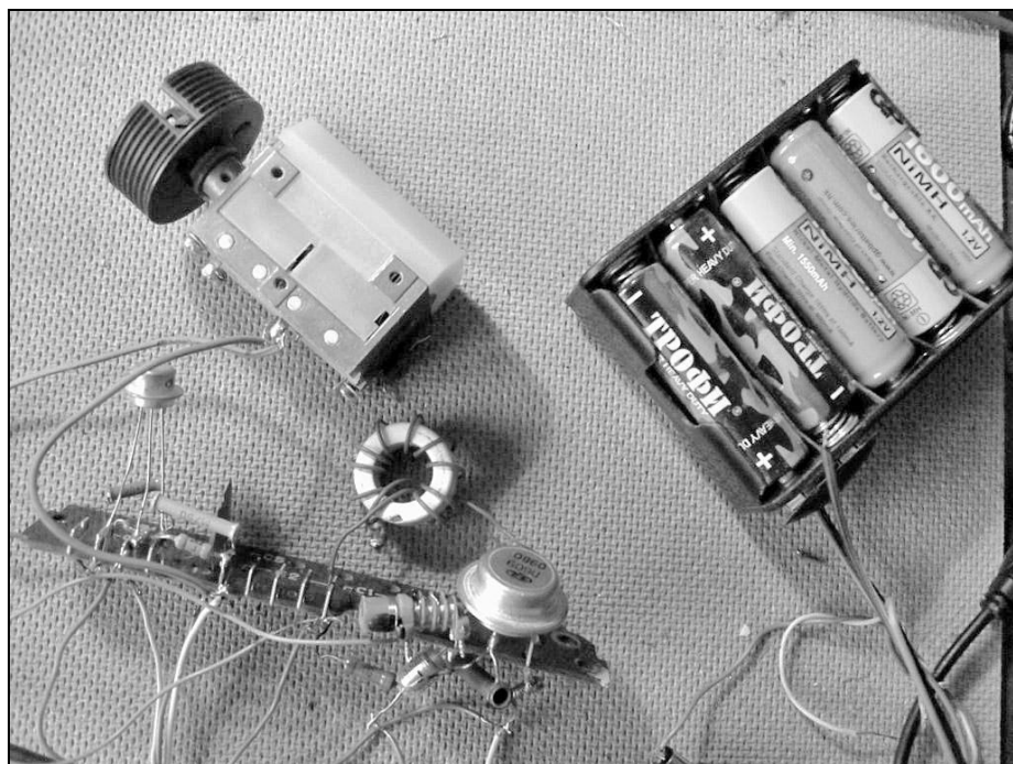
Yuri, UA3UAD - 100 mW TX (P416B + P605, Ge-pnp), G5RV
