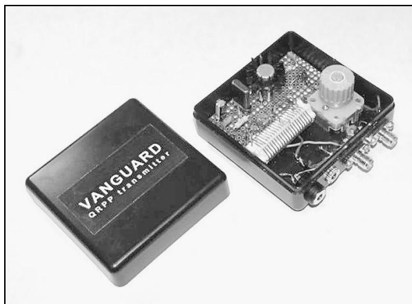
Petr, OK1DPX – 80 mW TX (AF114, Ge-pnp), dipole
